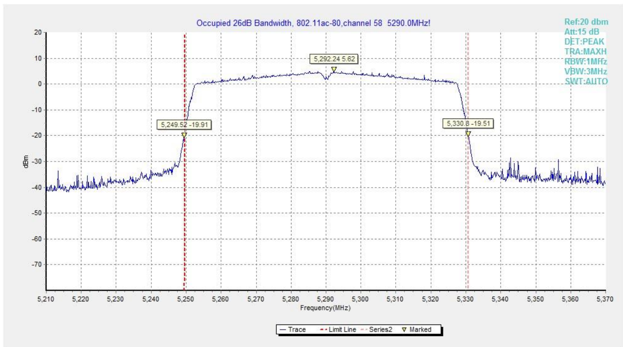
Fig.27 Occupied 26dB Bandwidth (802. 11ac-HT80, 5290MHz)
