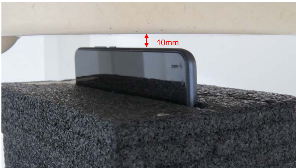
Picture 10: Right Edge, the distance from handset to the bottom of the Phantom is 10mm
