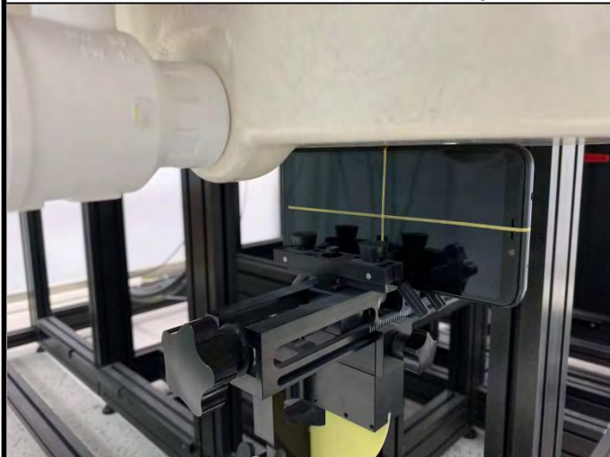
Left Side of EUT with 0 cm Gap
