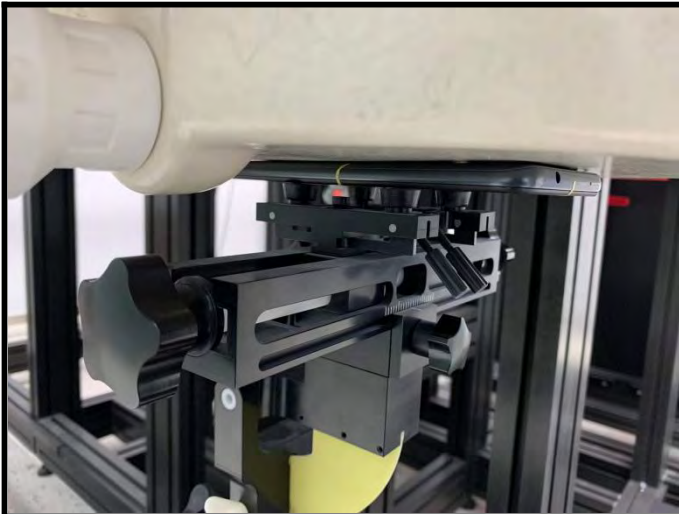
Rear Face of EUT with 0 cm Gap
