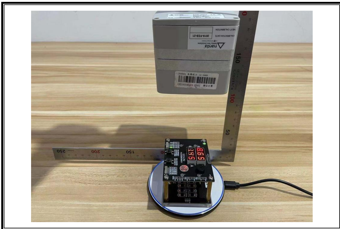
E-FILED AND H-FILED STRENGTH MEASUREMENT SETUP-E
