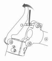
2-1 . Twist the bolt with 7 mm open end wrench little by little 2-2. Lock the folding mechanism to try if the handle stem still has a play
