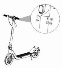
3. Using the 3mm Allen Wrench tighten the screws on both sides of steer tube.
