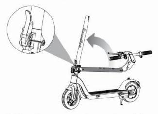
1. Place the scooter on the ground, push the kick stand down. Unfold the steer tube to vertical position and lock the folding mechanism.
