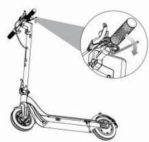
4. Adjust the hand brake to proper position, tighten the screw with 5mm Allen Wrench.
