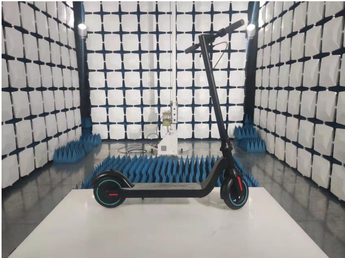
Above 1GHz for radiated emission test setup
