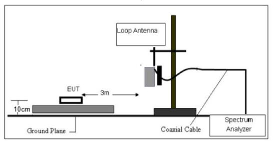
(B) Radiated Emission Test-Up Frequency 30MHz~1GHz
