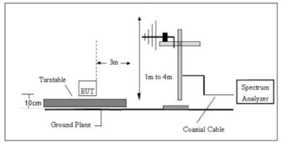
(C) Radiated Emission Test-Up Frequency Above 1GHz
