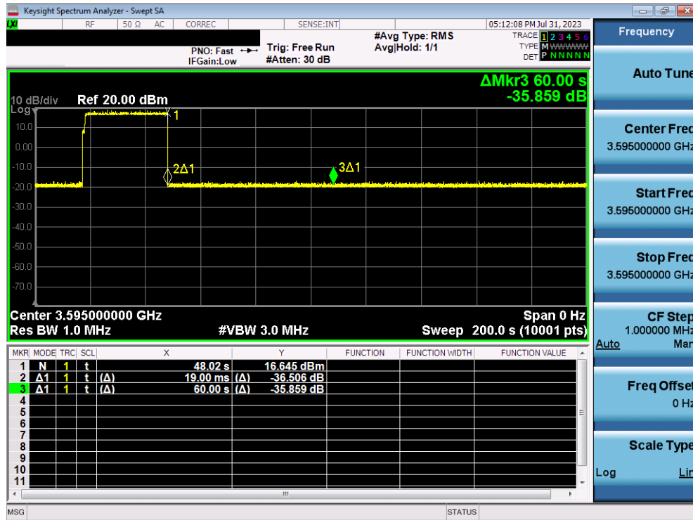
Plot 16. Conducted Measurement - RF transmission stops within 60s of SAS message. The SAS message is indicated by Marker 1 (X) (WINNF.FT.C.HBT.7)
