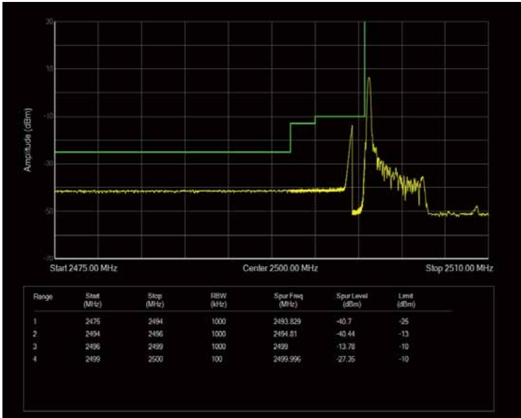
Band7 QAM16 BW=5MHz Channel=20775 RB Size=1 Position=#Max
