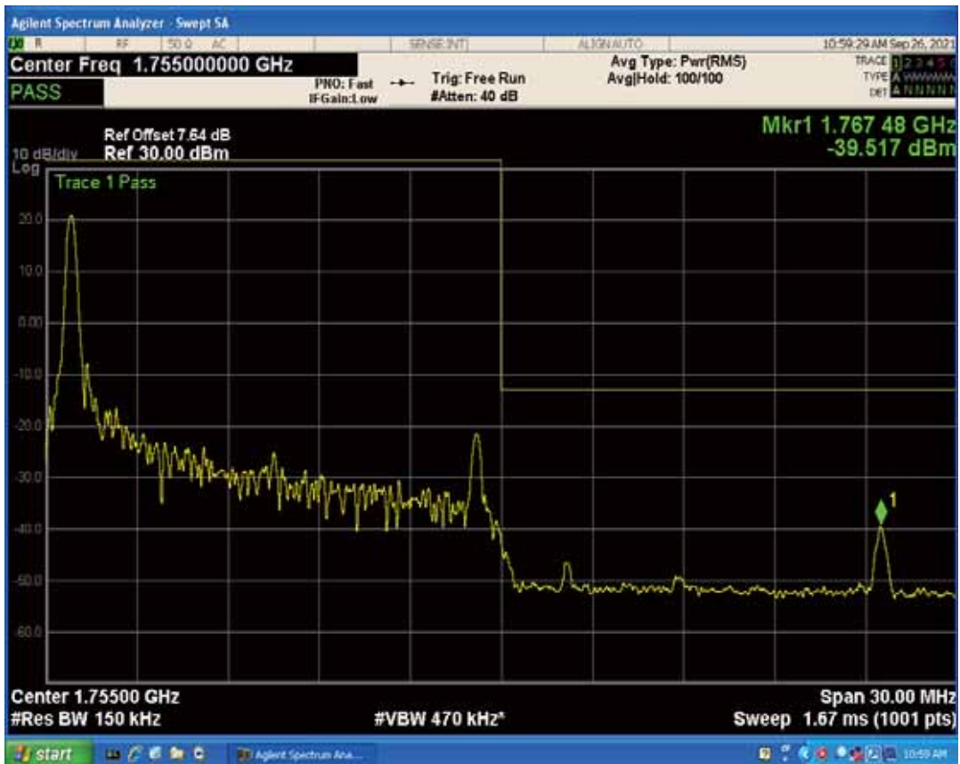
Band4 QPSK BW=15MHz Channel=20325 RB Size=75 Position=#0
