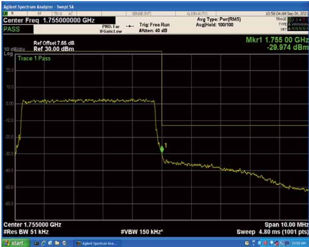
Band4 QPSK BW=10MHz Channel=20000 RB Size=1 Position=#0
