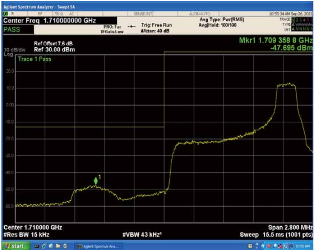
Band4 QAM16 BW=1.4MHz Channel=19957 RB Size=1 Position=#0
