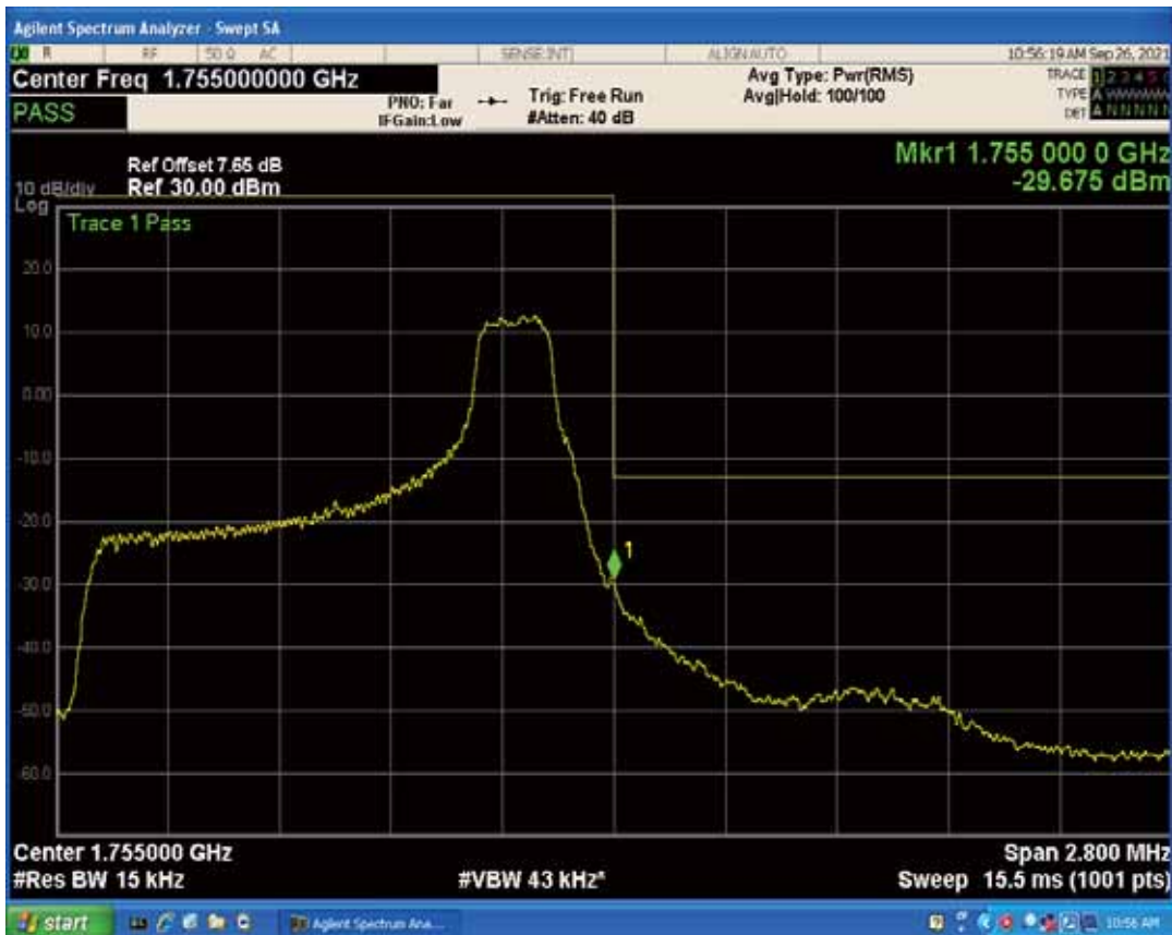
Band4 QPSK BW=3MHz Channel=19965 RB Size=1 Position=#0
