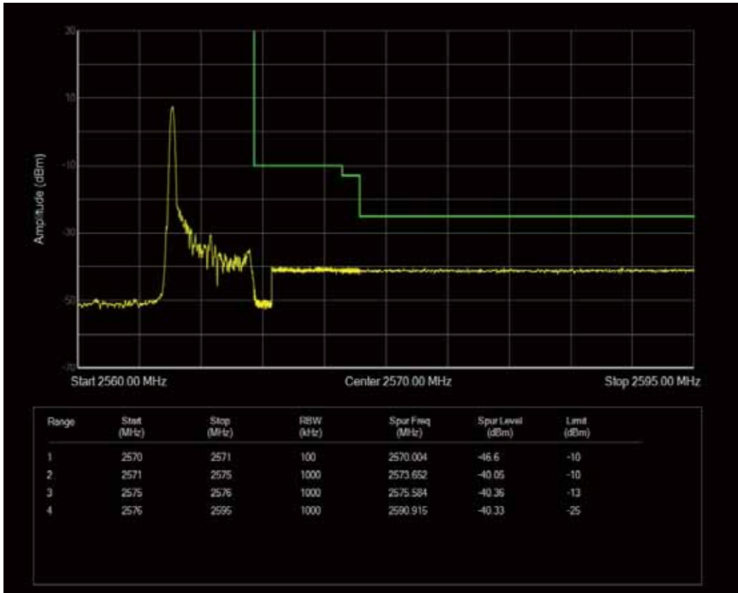
Band7 QAM16 BW=5MHz Channel=21425 RB Size=1 Position=#Max
