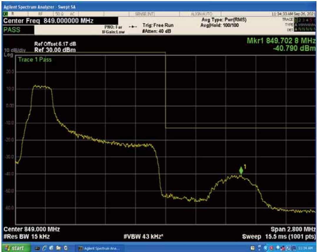
Band5 QAM16 BW=1.4MHz Channel=20643 RB Size=1 Position=#Max
