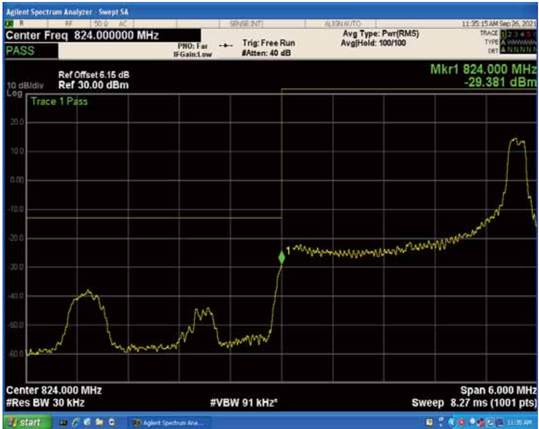
Band5 QPSK BW=3MHz Channel=20635 RB Size=1 Position=#0
