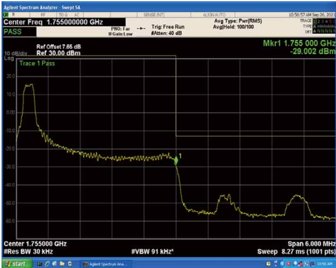
Band4 QPSK BW=3MHz Channel=20385 RB Size=15 Position=#0
