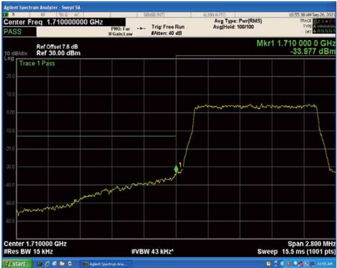
Band4 QAM16 BW=1.4MHz Channel=19957 RB Size=1 Position=#Max
