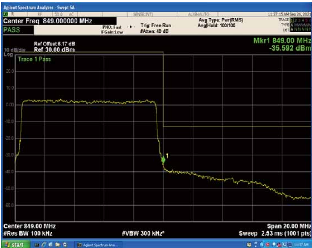
Band5 QAM16 BW=10MHz Channel=20600 RB Size=1 Position=#0
