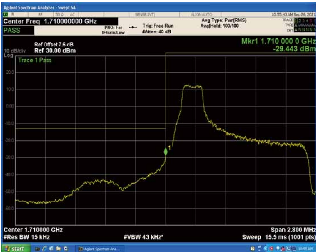
Band4 QPSK BW=1.4MHz Channel=19957 RB Size=6 Position=#0
