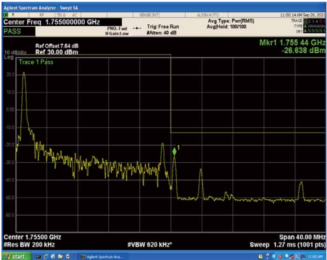
Band4 QPSK BW=20MHz Channel=20300 RB Size=1 Position=#Max
