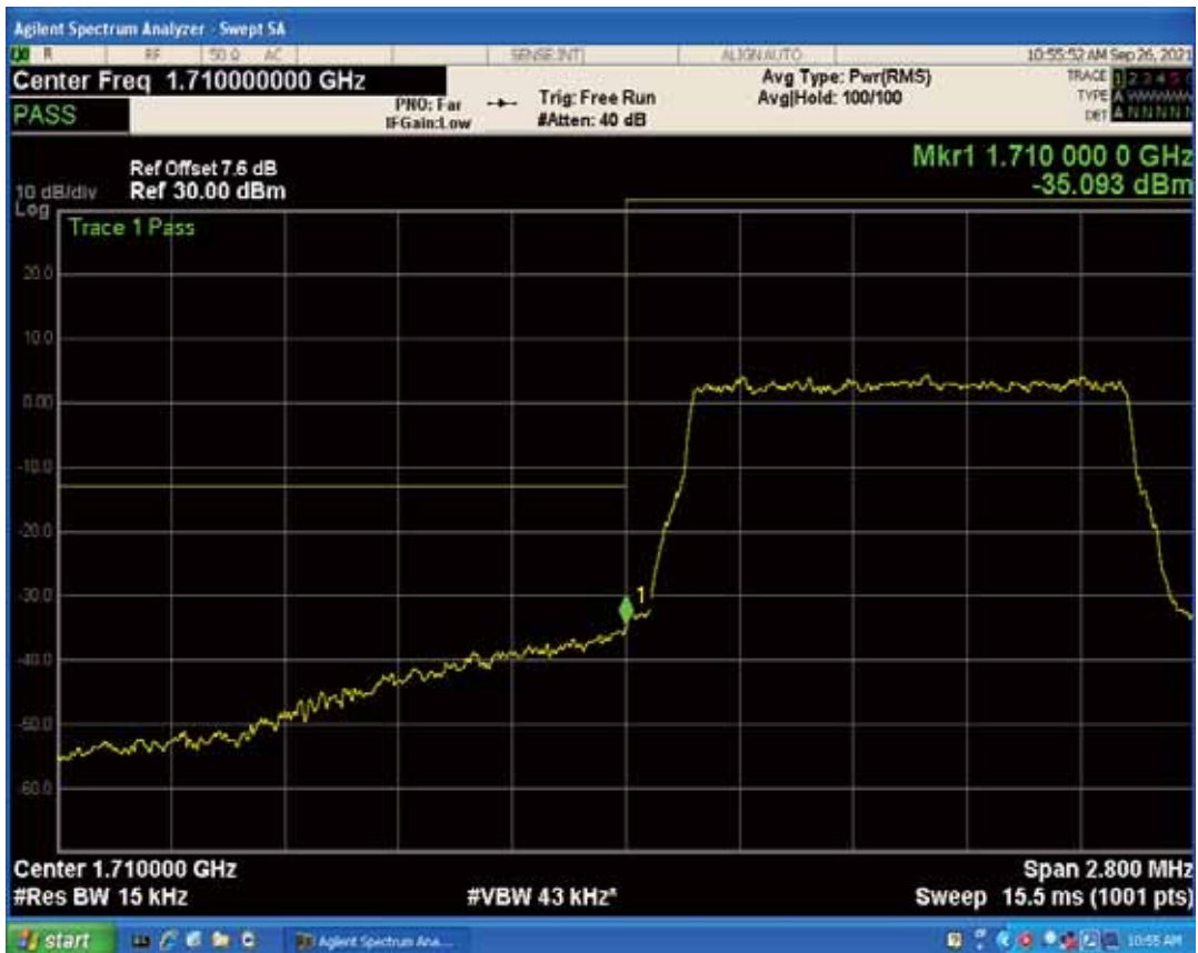
Band4 QPSK BW=1.4MHz Channel=20393 RB Size=1 Position=#Max
