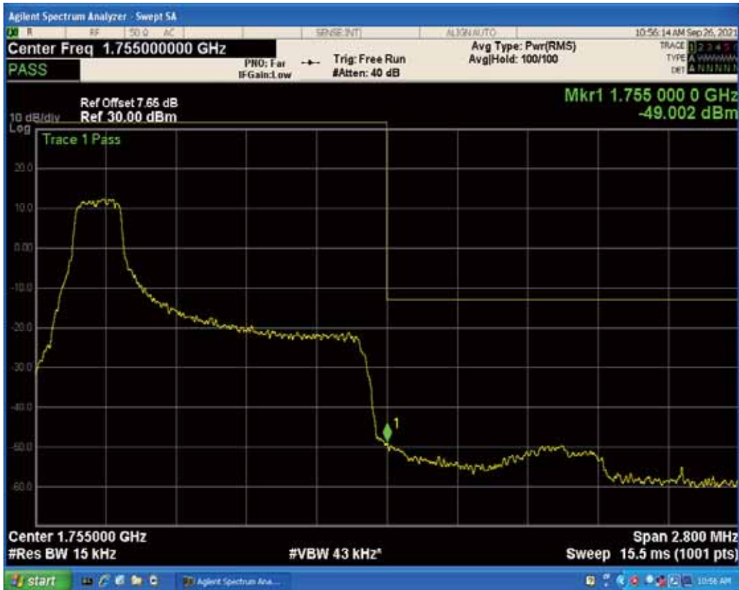
Band4 QAM16 BW=1.4MHz Channel=20393 RB Size=1 Position=#Max
