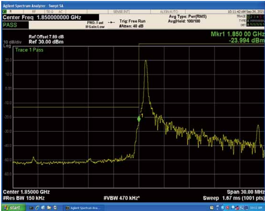
Band2 QAM16 BW=10MHz Channel=19150 RB Size=50 Position=#0
