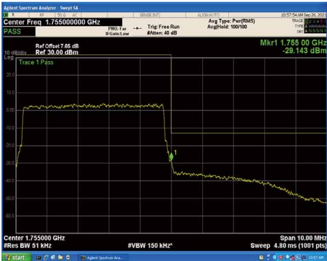
Band4 QAM16 BW=5MHz Channel=20375 RB Size=1 Position=#0
