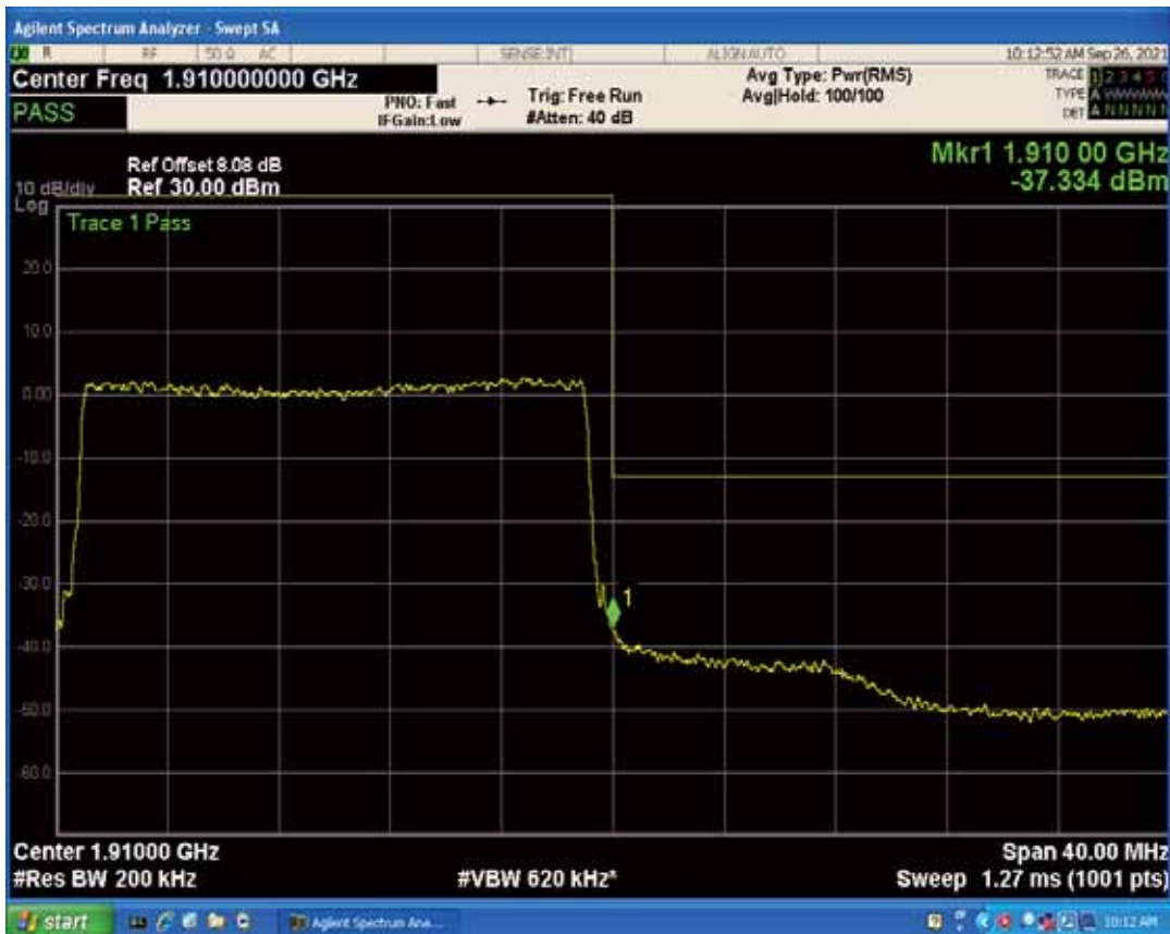
Band2 QAM16 BW=20MHz Channel=19100 RB Size=1 Position=#0
