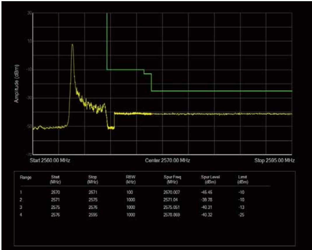
Band7 QPSK BW=5MHz Channel=21425 RB Size=25 Position=#0
