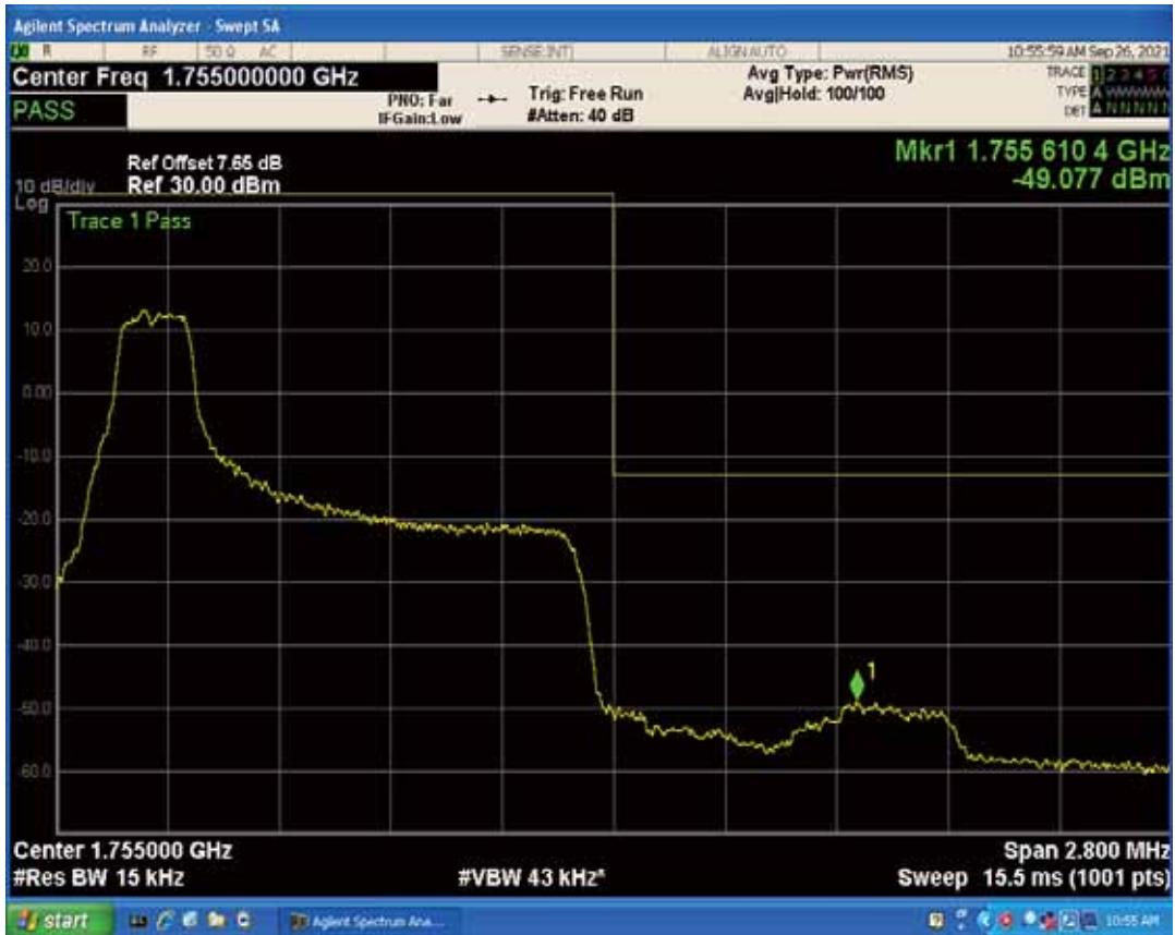
Band4 QAM16 BW=1.4MHz Channel=19957 RB Size=6 Position=#0
