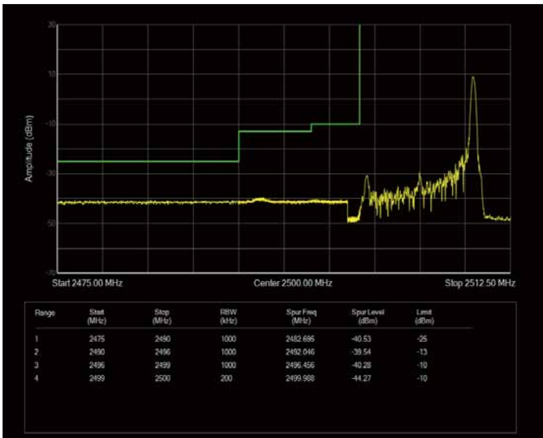
Band7 QAM16 BW=10MHz Channel=20800 RB Size=50 Position=#0
