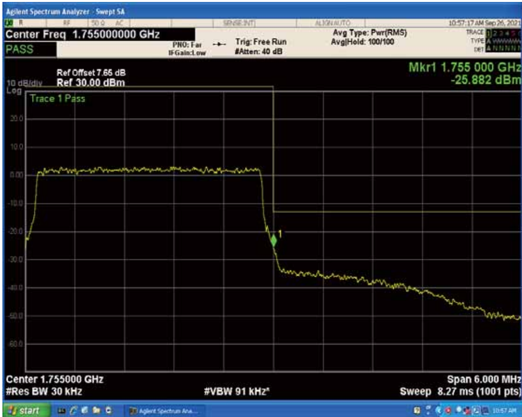
Band4 QPSK BW=5MHz Channel=19975 RB Size=1 Position=#Max
