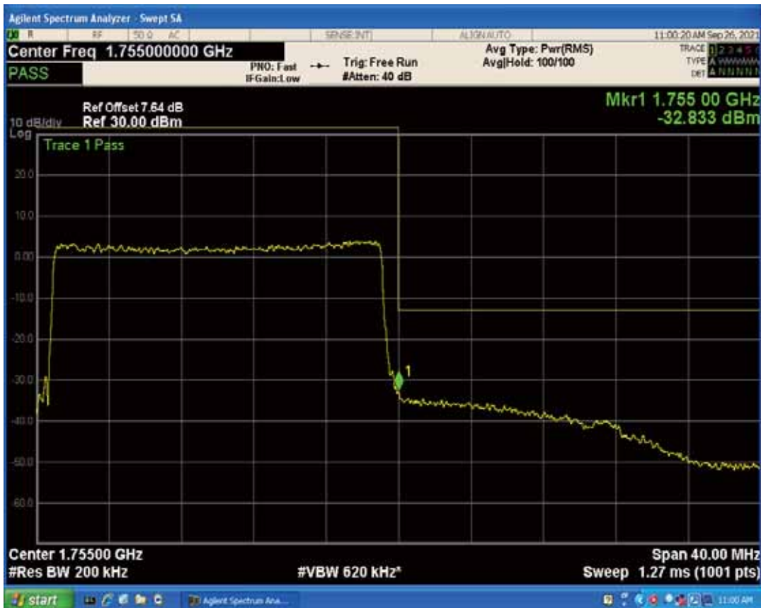
Band4 QAM16 BW=20MHz Channel=20300 RB Size=1 Position=#0
