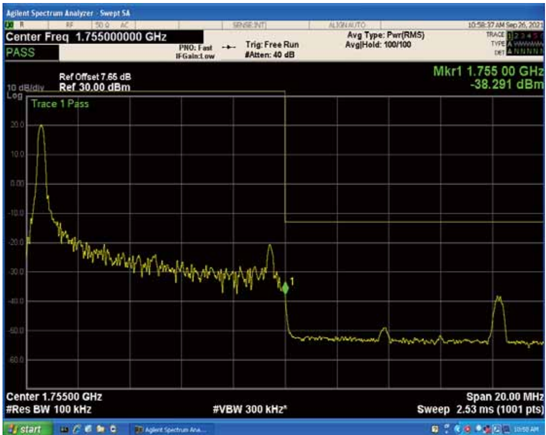
Band4 QPSK BW=10MHz Channel=20350 RB Size=50 Position=#0
