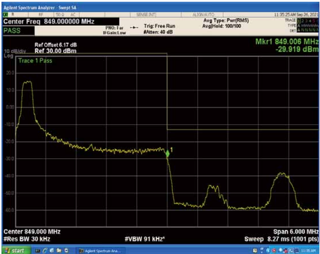
Band5 QPSK BW=3MHz Channel=20635 RB Size=15 Position=#0
