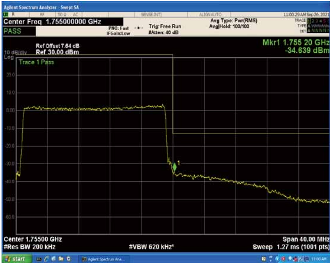
Band5 QPSK BW=1.4MHz Channel=20407 RB Size=1 Position=#0
