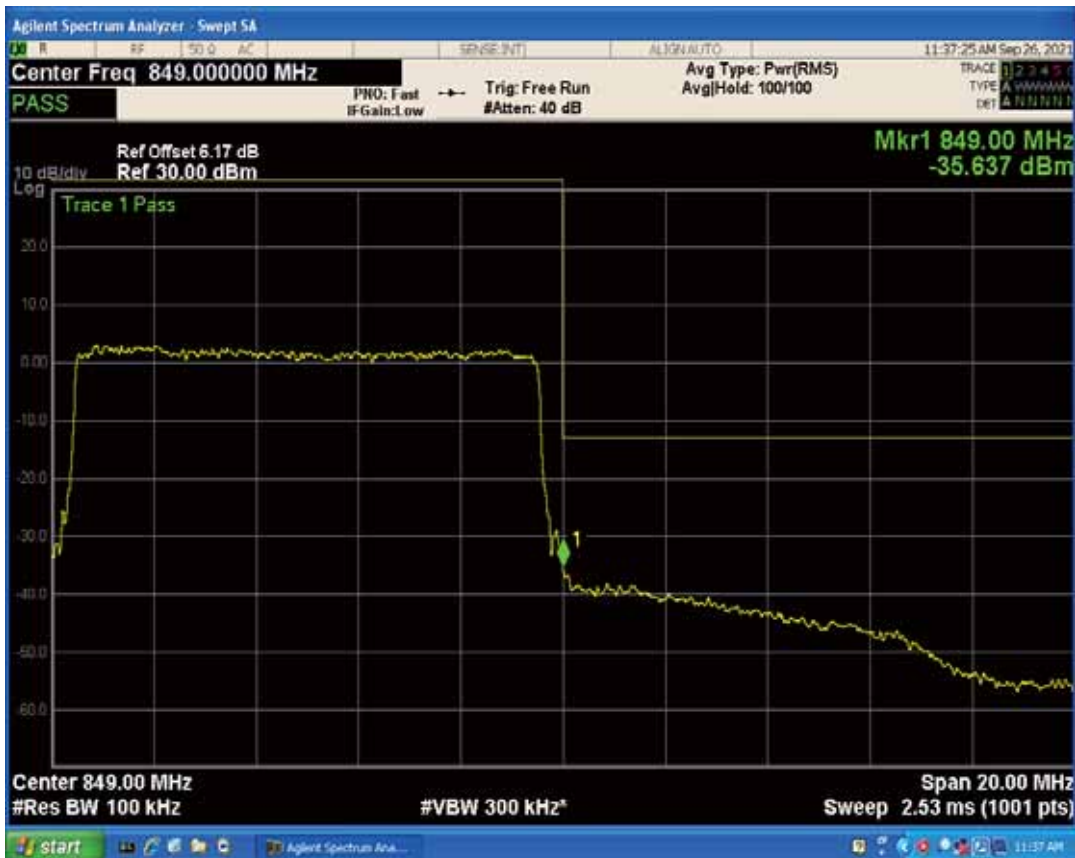
Band5 QAM16 BW=10MHz Channel=20600 RB Size=1 Position=#Max
