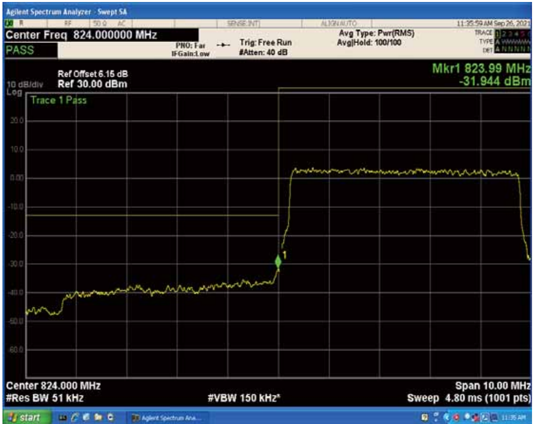
Band5 QPSK BW=5MHz Channel=20425 RB Size=1 Position=#Max
