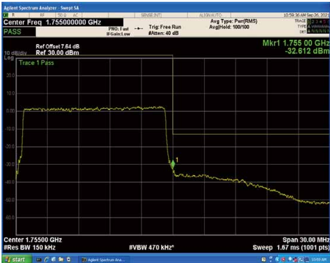
Band4 QPSK BW=20MHz Channel=20050 RB Size=1 Position=#Max
