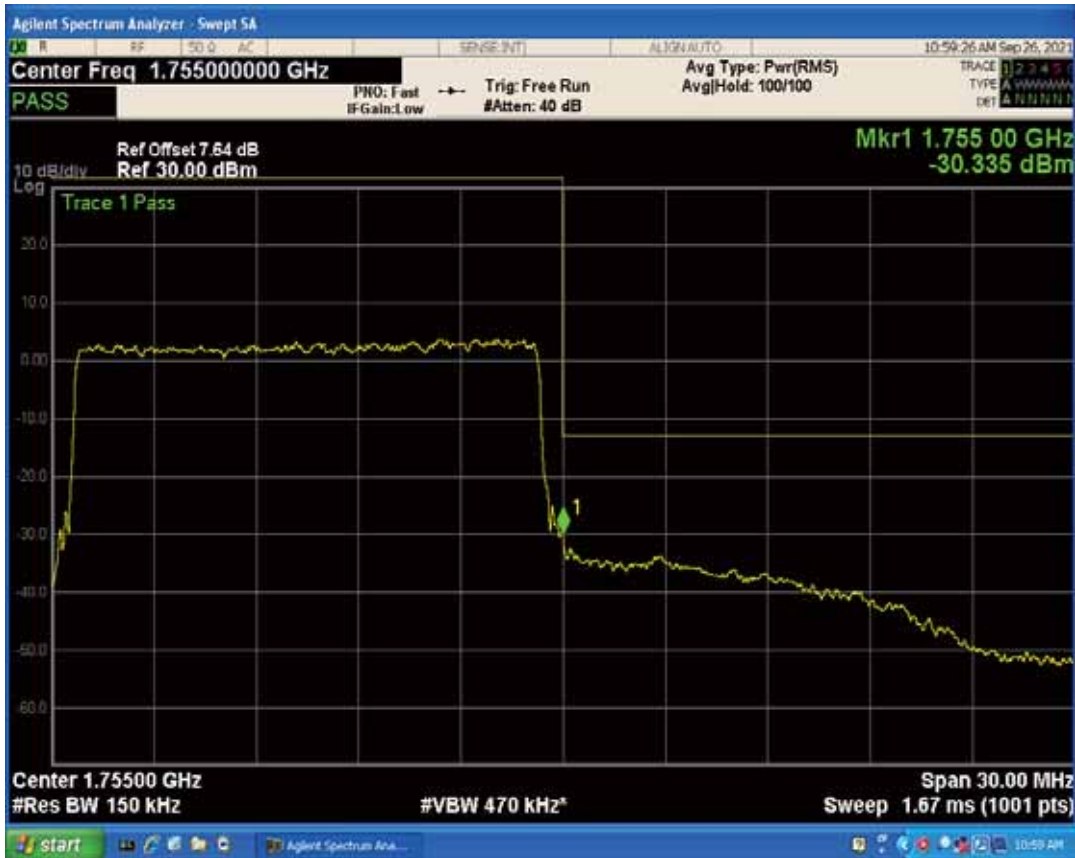
Band4 QAM16 BW=15MHz Channel=20325 RB Size=1 Position=#Max
