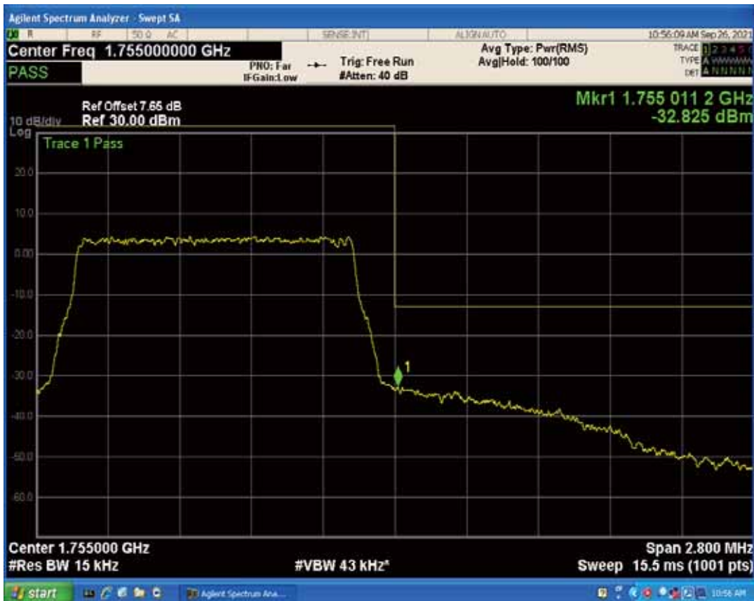
Band4 QAM16 BW=1.4MHz Channel=20393 RB Size=1 Position=#0
