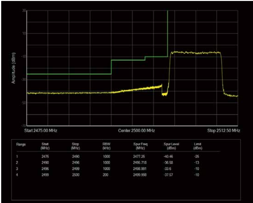
Band7 QAM16 BW=10MHz Channel=20800 RB Size=1 Position=#Max
