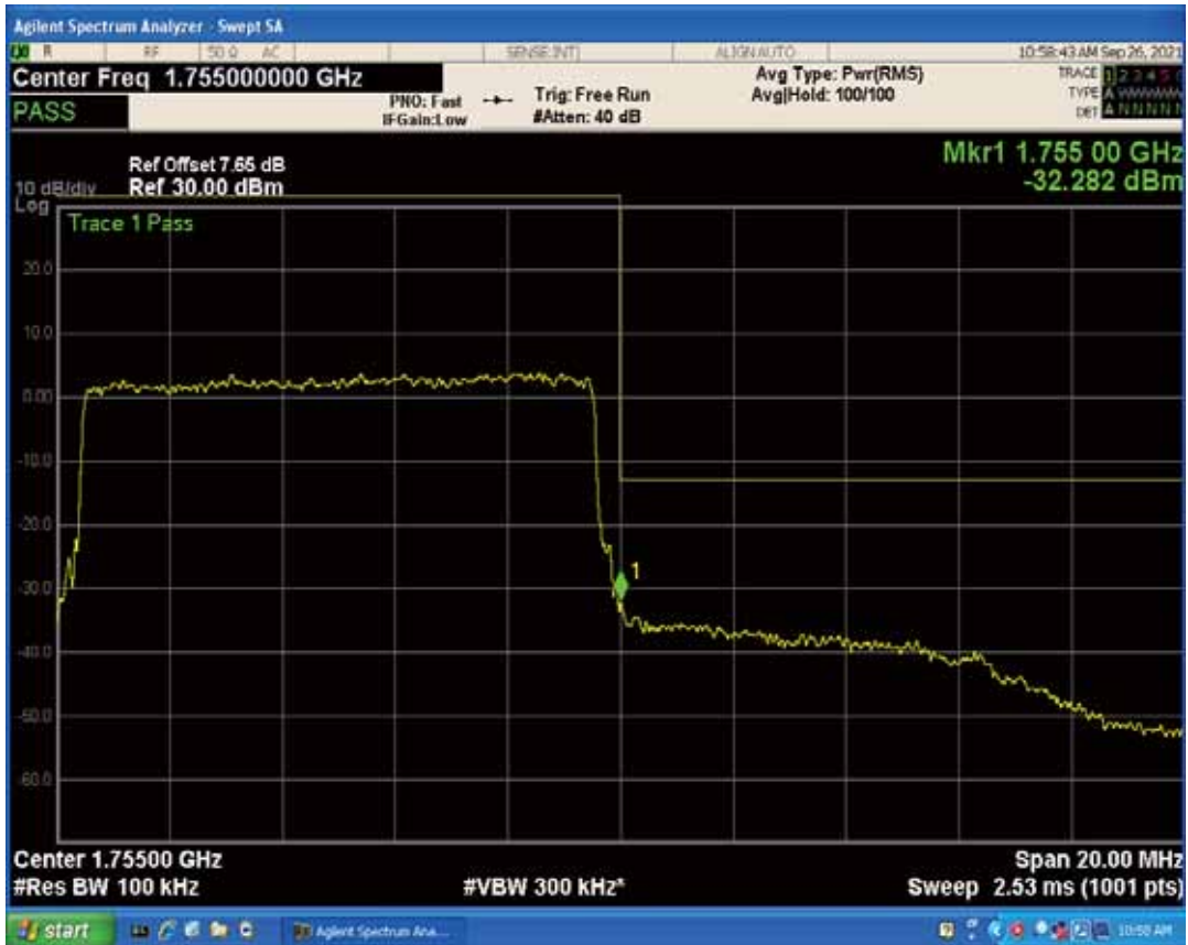
Band4 QPSK BW=10MHz Channel=20350 RB Size=1 Position=#Max
