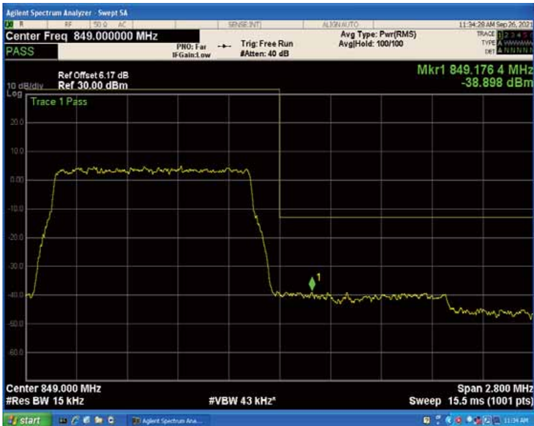
Band5 QAM16 BW=1.4MHz Channel=20643 RB Size=1 Position=#0
