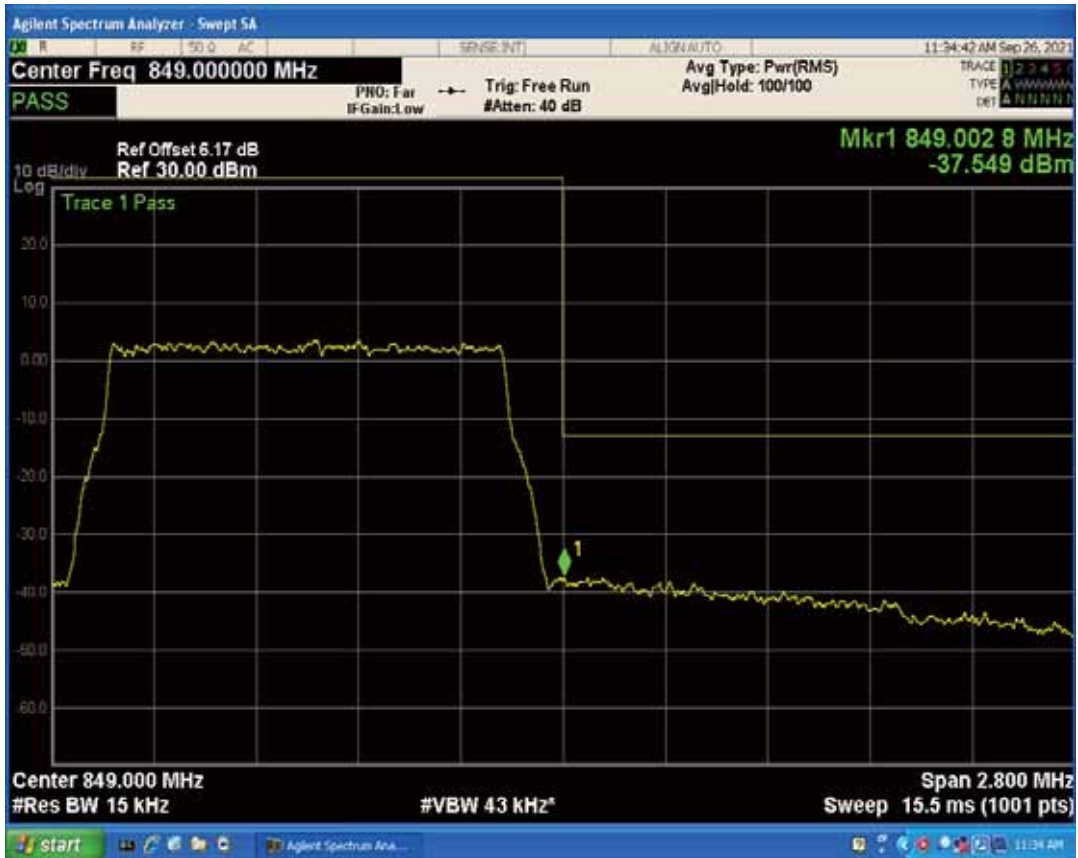
Band5 QPSK BW=3MHz Channel=20415 RB Size=1 Position=#0
