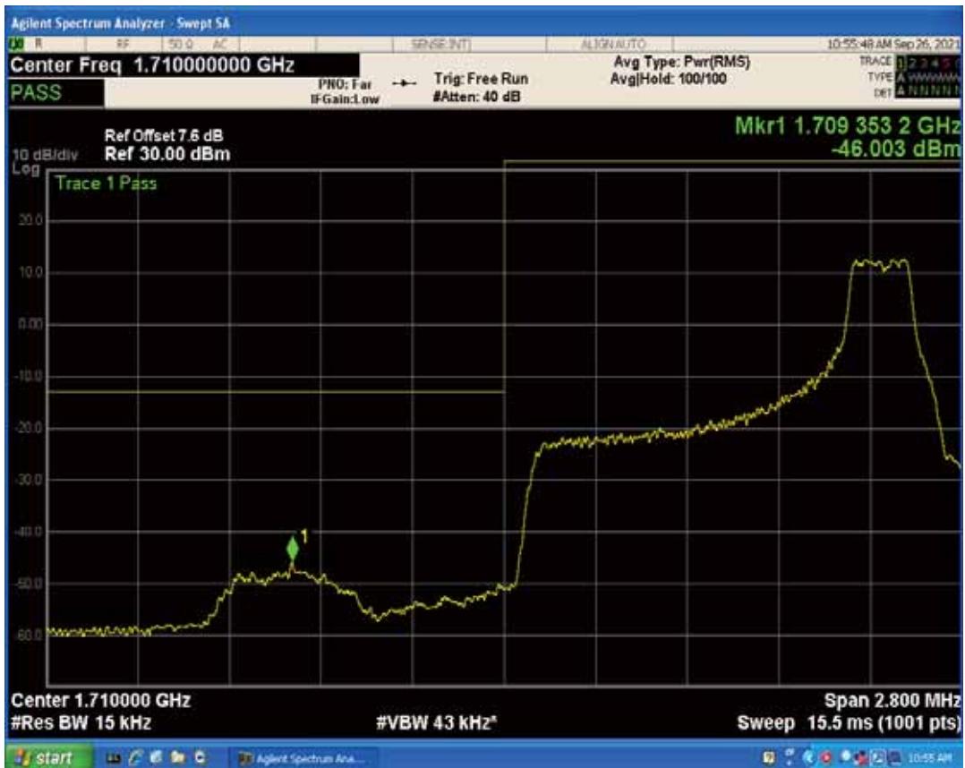
Band4 QPSK BW=1.4MHz Channel=20393 RB Size=1 Position=#0
