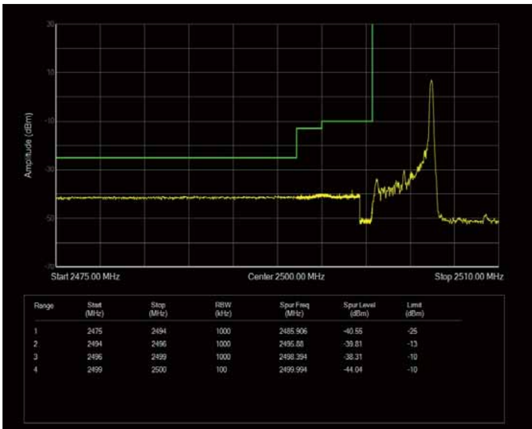
Band7 QAM16 BW=5MHz Channel=20775 RB Size=25 Position=#0
