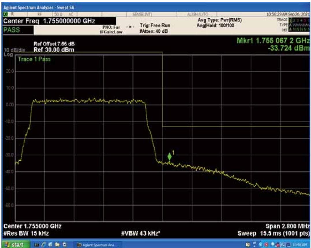
Band4 QPSK BW=3MHz Channel=19965 RB Size=1 Position=#Max
