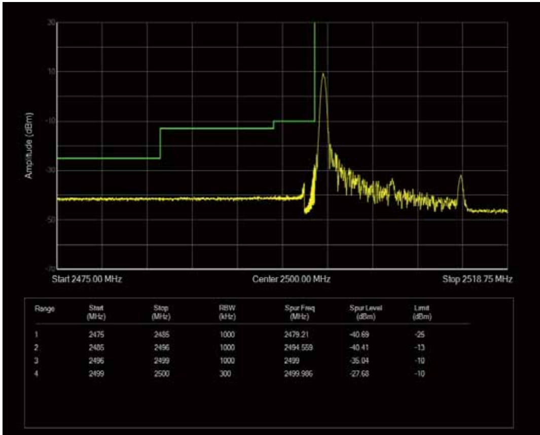
Band7 QAM16 BW=15MHz Channel=20825 RB Size=1 Position=#Max
