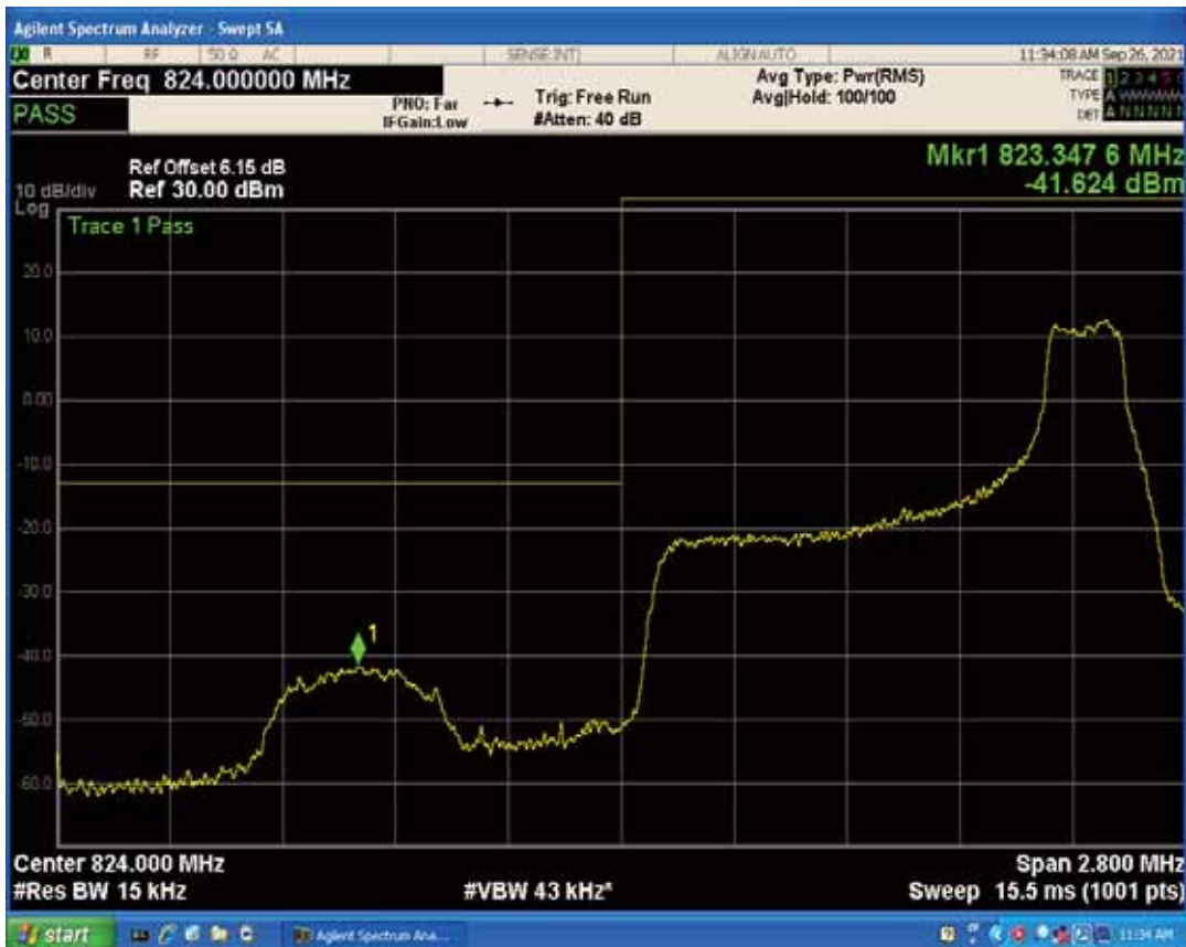
Band5 QPSK BW=1.4MHz Channel=20643 RB Size=1 Position=#0
