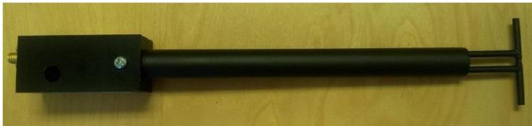
Figure 1 – MVG COMOSAR Validation Dipole
