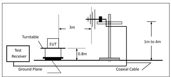
(c) For radiated emissions above 1000MHz
