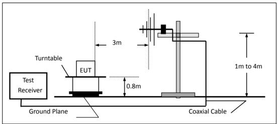
(c) For radiated emissions above 1000MHz
