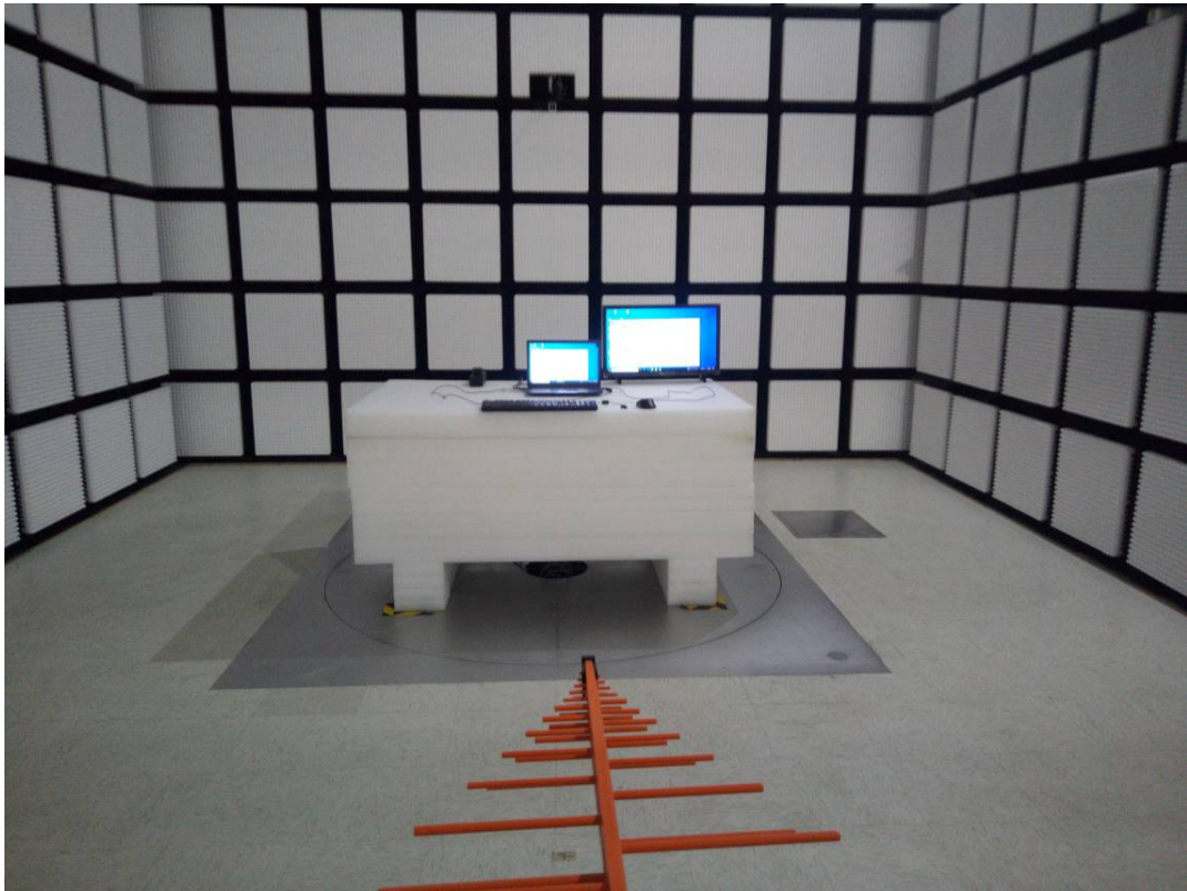
Radiated Emission Above 1GHz View
