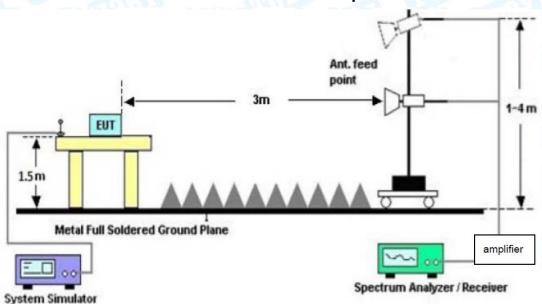
**Above 1GHz Test Setup**
