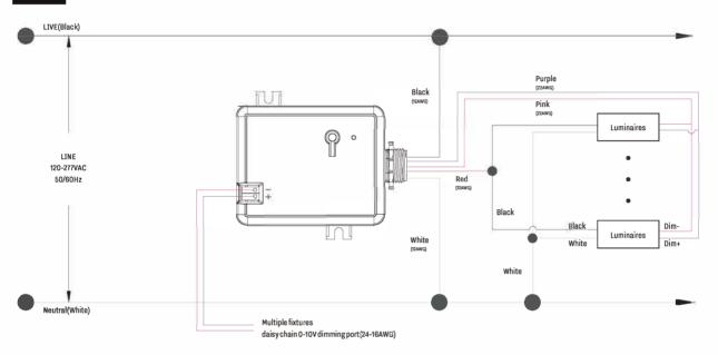
Note: PPA104S MAX Load 20A, Sink Current Max.48.5mA of the dimming port.
