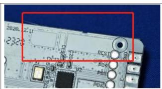
The antenna is PCB antenna.
