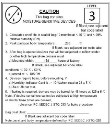
The module Must go through 125  $^{\circ}$ C baking for at least 9 hours before SMT AND IR reflow process!
