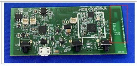
The antenna is PCB antenna. The best case gain of the antenna is 3.3dBi.
