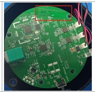
The antenna is PCB antenna. The best case gain of the antenna is 3.3dBi.
