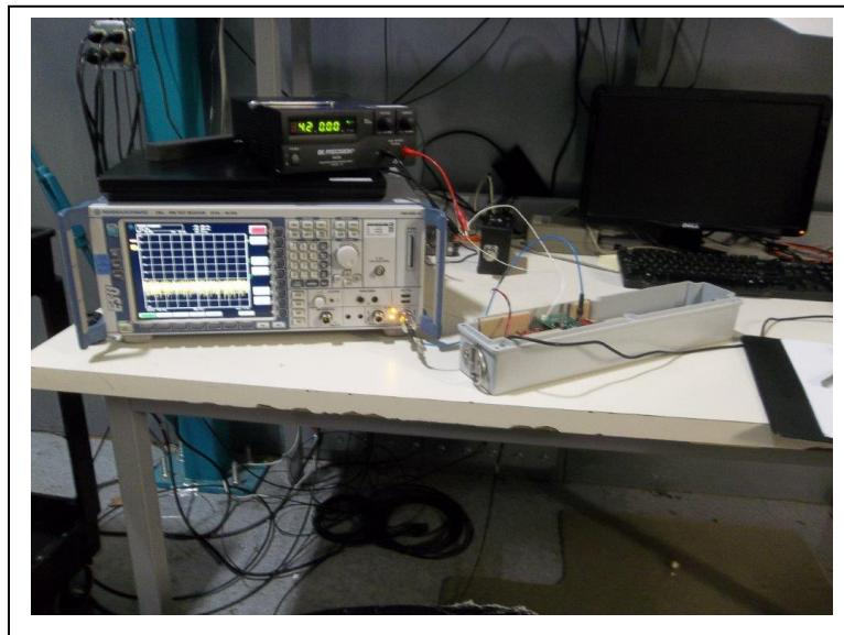
**Conducted Output Power, Peak Power Spectral Density,
