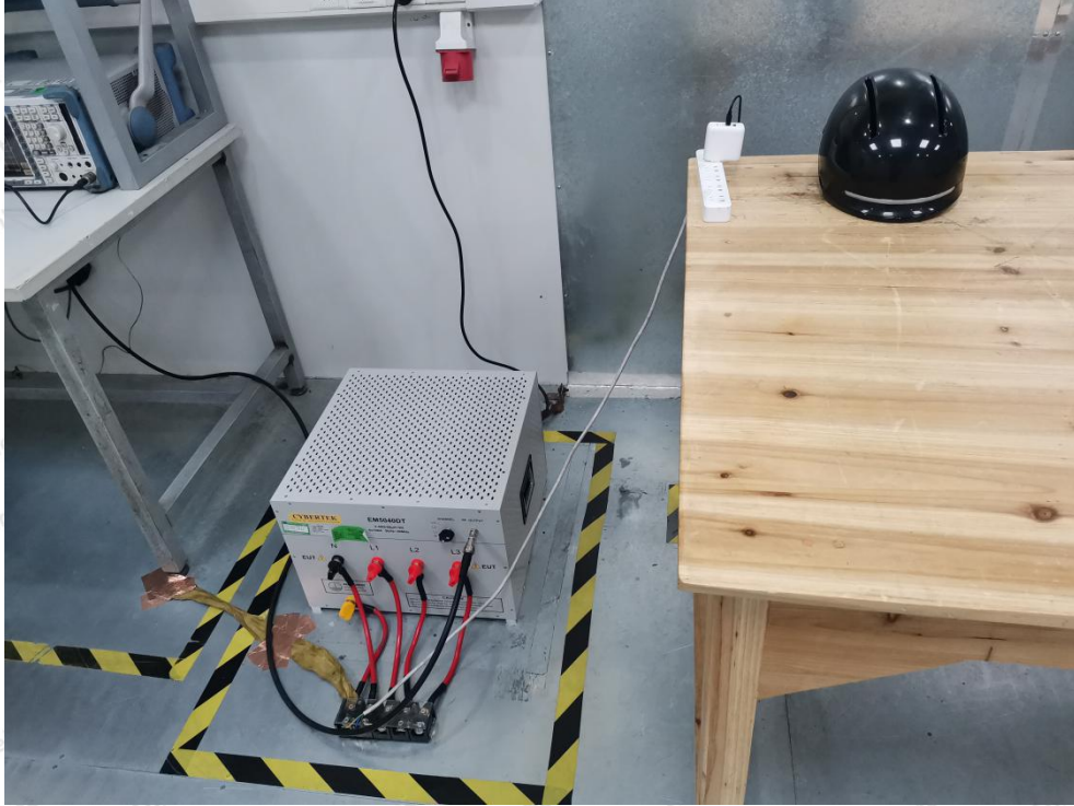
Photo of Conducted Emission Measurement
