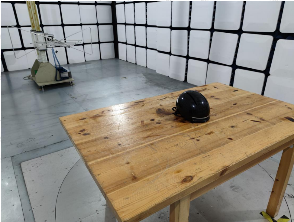
Photo of Radiation Emission Test
