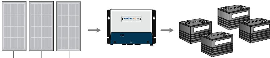
The charge controller controls how the batteries are charged by the DC source (the PV array).
