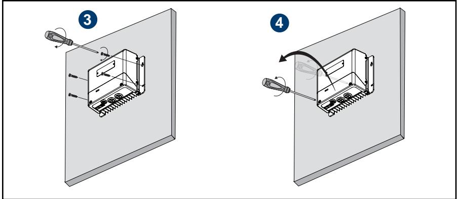
**3** Using the provided mounting screws, secure the charge controller on the wall.
