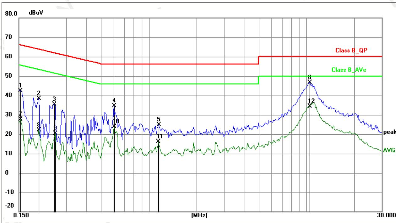
Remark: Factor = Insertion Loss + Cable Loss, Result = Reading + Factor, Margin = Result – Limit.
