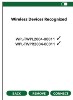
Wireless pulsers show up as left and right and both must be selected. Press connect to pair.
