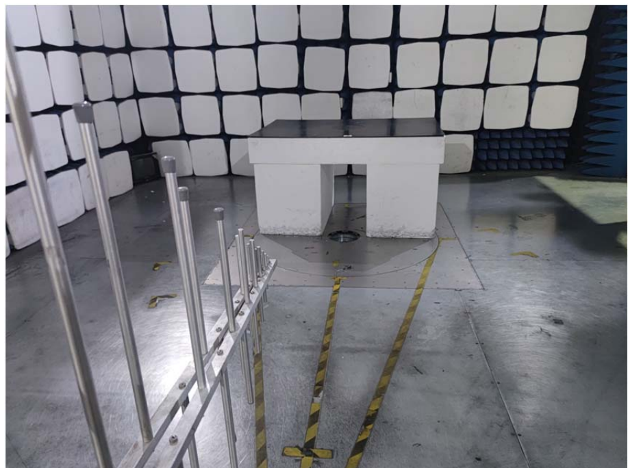
Radiation Emission Test Setup (30MHz to 1GHz)
