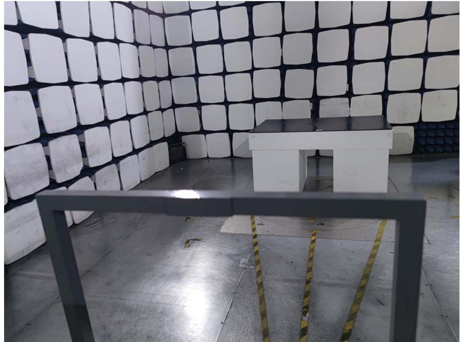
Radiation Emission Test Setup (Below 30MHz)
