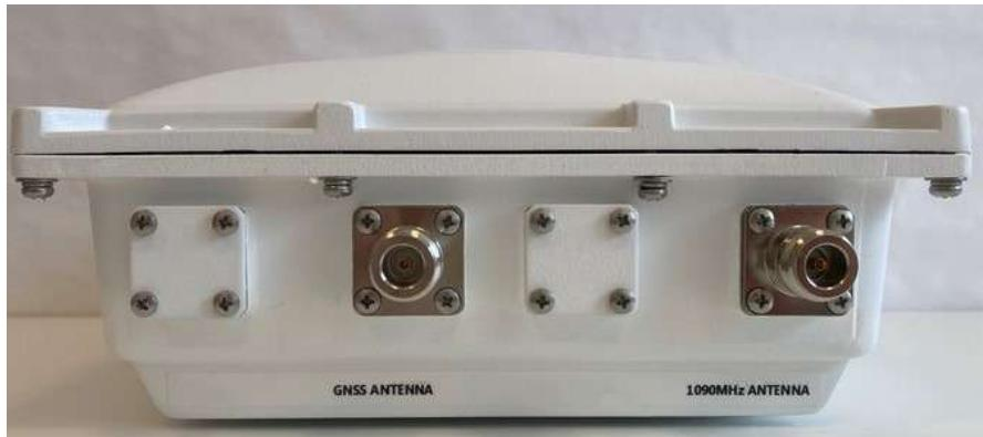
Screw the GPS antenna and the 1090 MHz antenna on their N connectors, according to indications. For a 1090 MHz antenna, use a male-to-male N-type adapter. The picture below shows properly installed antennas:
