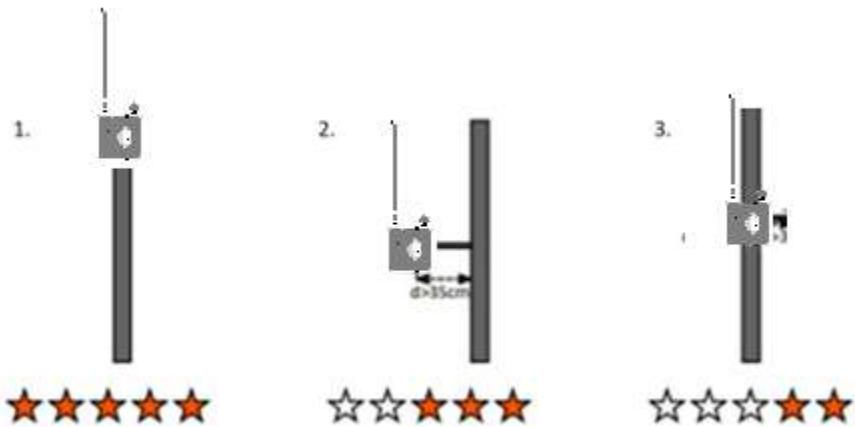
The G-1090 receiver should be installed on the top of a pole, in a way that the pole itself is not hiding the antennas (1.). If this is not possible, it is strongly recommended to place the antennas at least 35 cm of distance from the pole itself (2. and 3.), in order to avoid reflections of signals. Installing the receiver behind another device or too close to an emitting device is strongly not recommended, as it will lower the reception capability of the G-1090.
