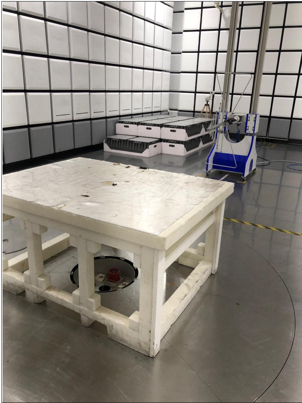
Frequency Range-Right Earphone < 30MHz~1GHz >
