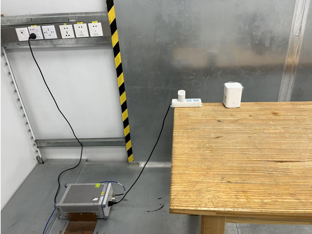
AC Power Line Conducted Emission
