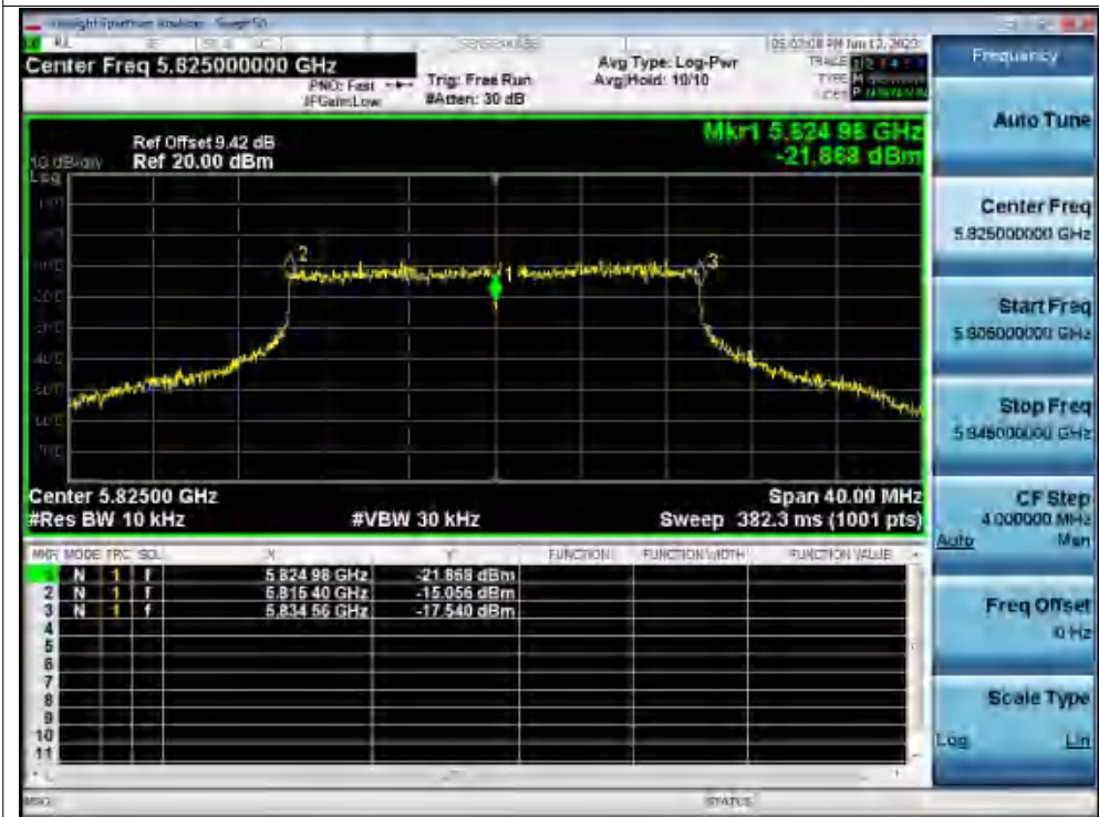
Freq. Stability 50C 120V ax20 5825MHz Ant1 0 Minutes
