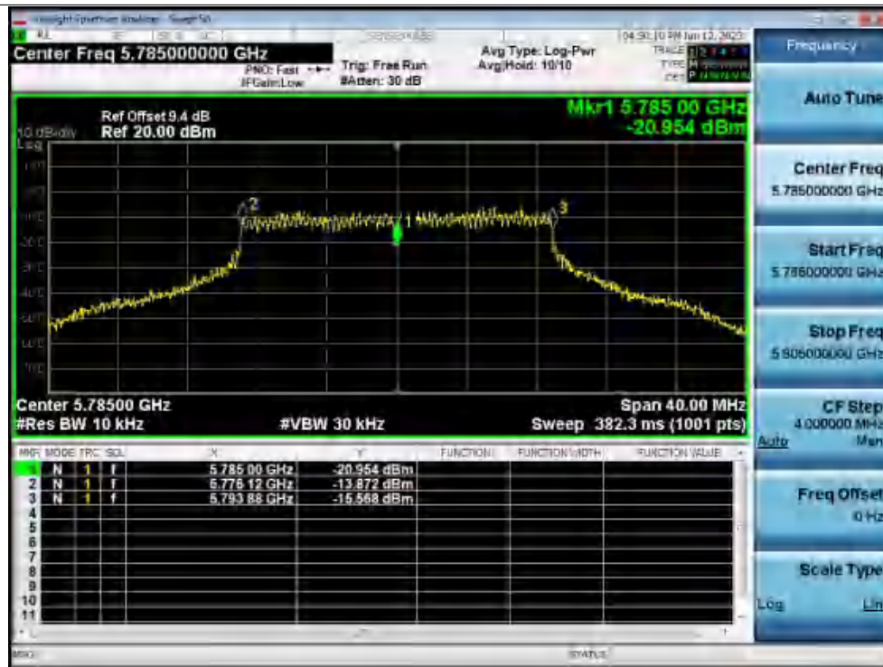
Freq. Stability 30C 120V ac20 5785MHz Ant1 0 Minutes
