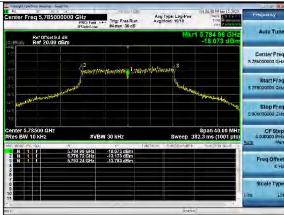
Freq. Stability 30C 120V a 5785MHz Ant1 0 Minutes
