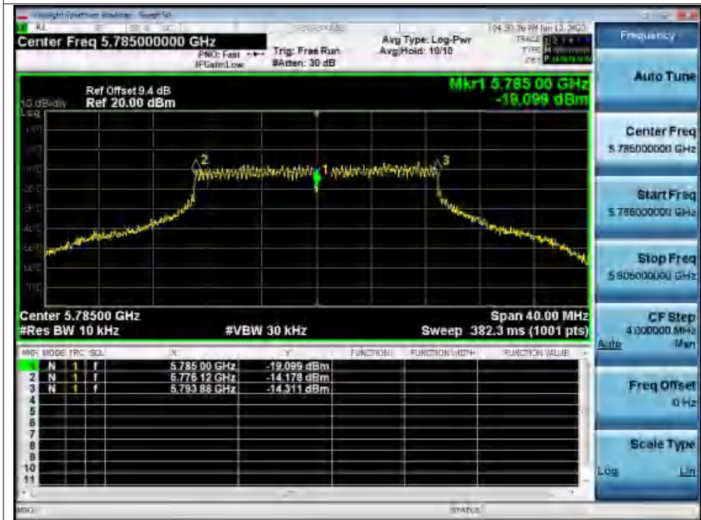
Freq. Stability 50C 120V ac20 5785MHz Ant1 0 Minutes
