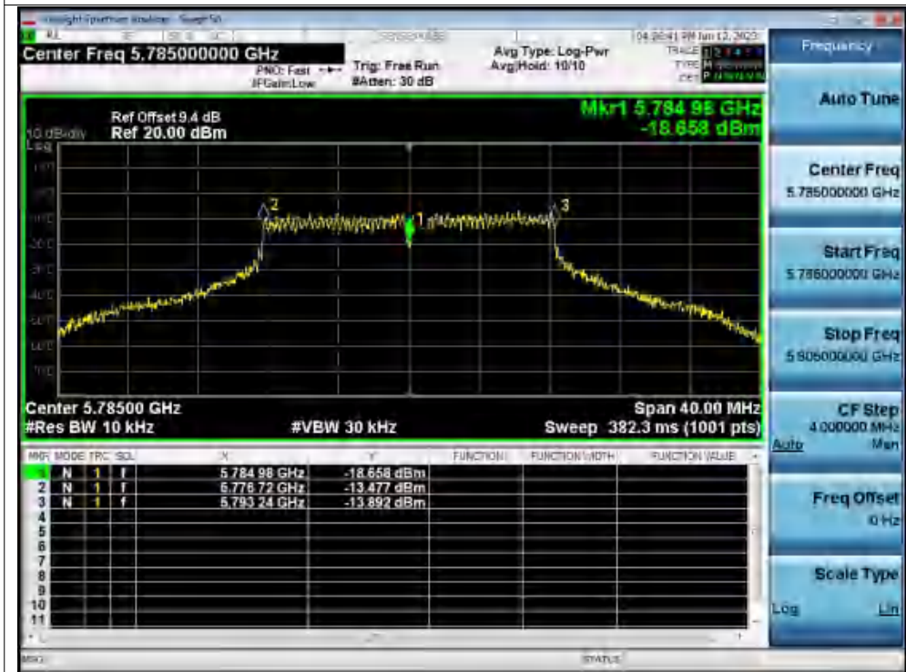
Freq. Stability 0C 120V a 5785MHz Ant1 0 Minutes
