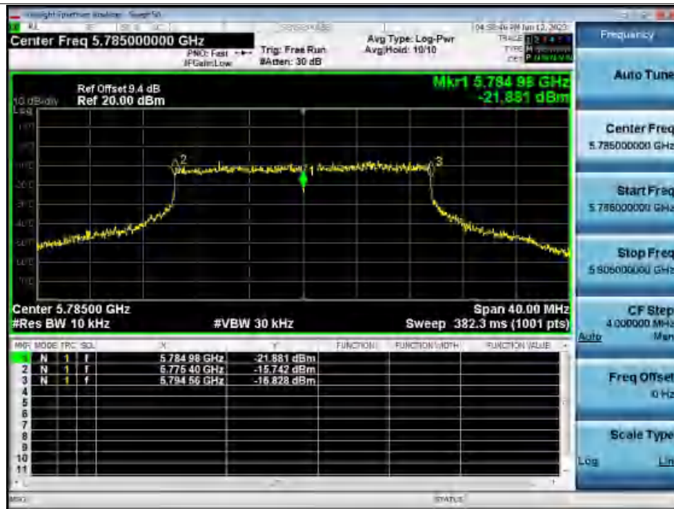
Freq. Stability 0C 120V ax20 5785MHz Ant1 0 Minutes
