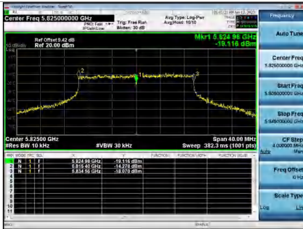
Freq. Stability 0C 120V ax20 5825MHz Ant1 0 Minutes
