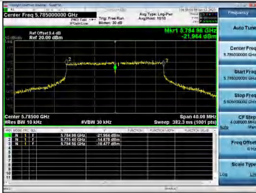
Freq. Stability 30C 120V ax20 5785MHz Ant1 0 Minutes
