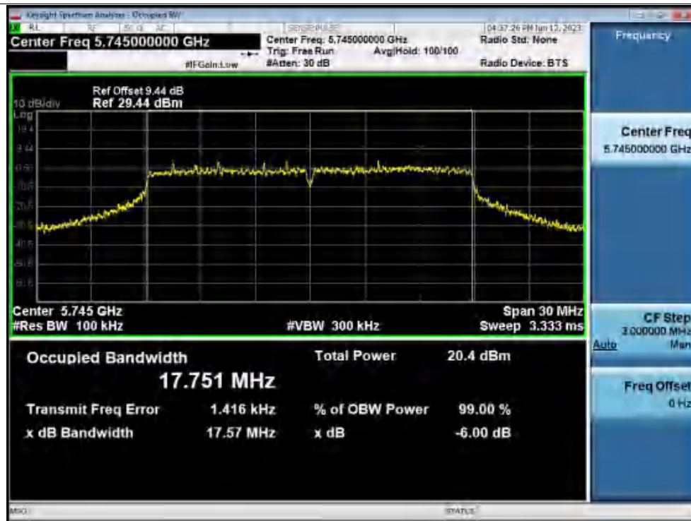
-6dB Bandwidth NVNT n20 5745MHz Ant1
