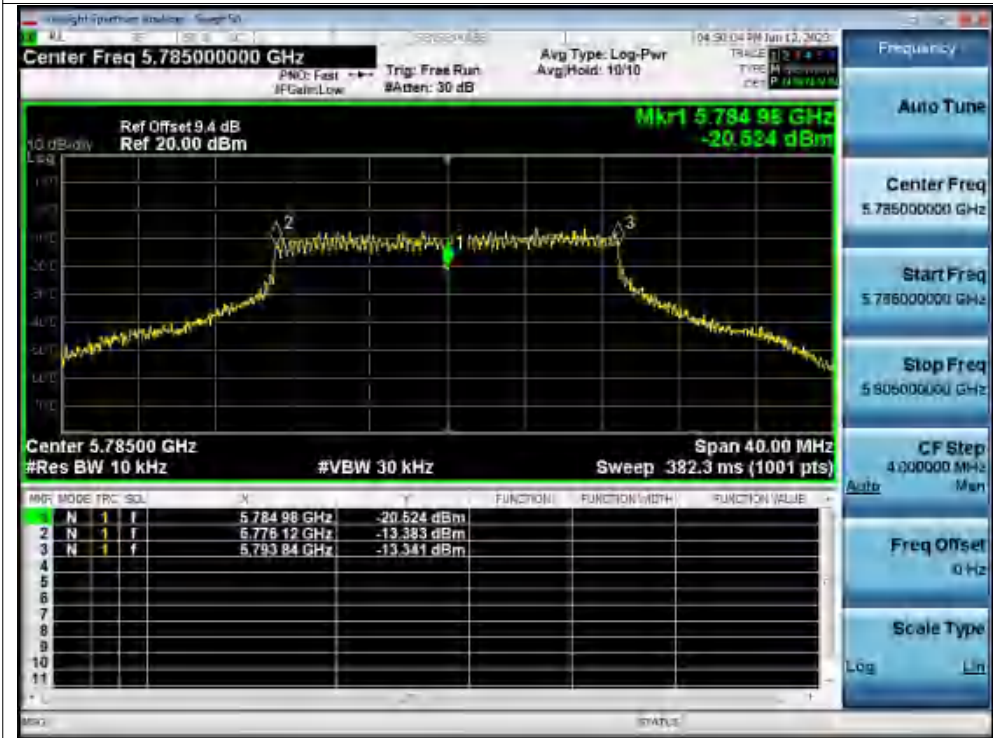
Freq. Stability 0C 120V ac20 5785MHz Ant1 0 Minutes
