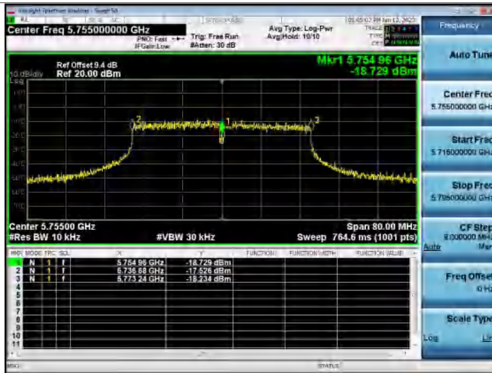
Freq. Stability 30C 120V n40 5755MHz Ant1 0 Minutes
