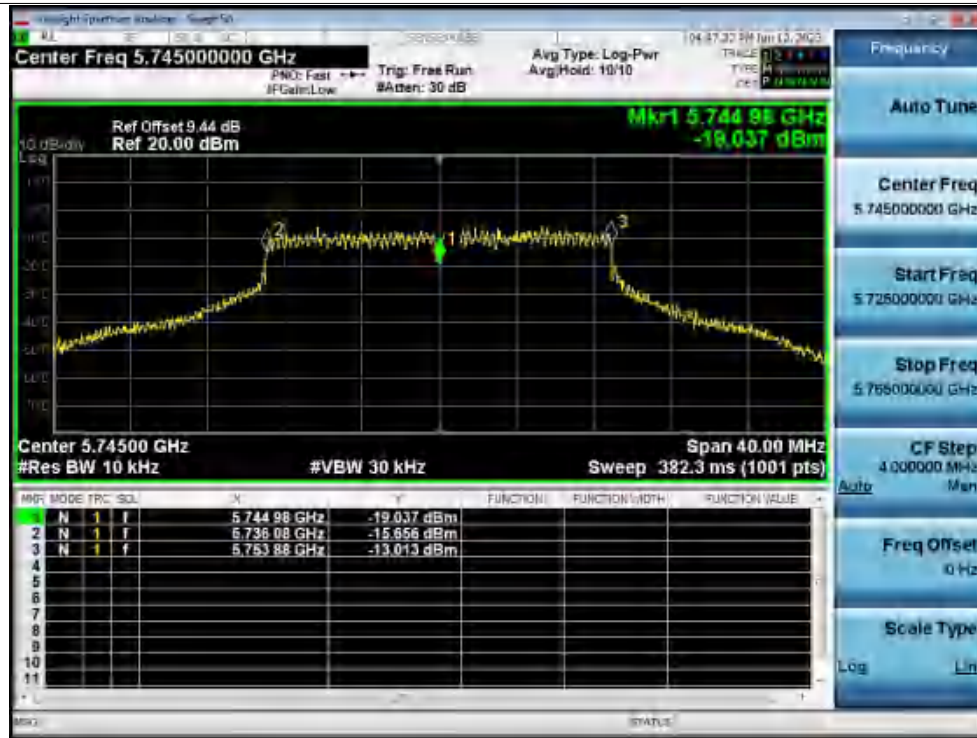
Freq. Stability 50C 120V ac20 5745MHz Ant1 0 Minutes
