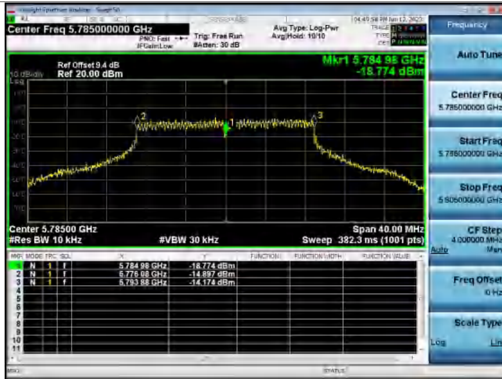
Freq. Stability 0C 120V ac20 5785MHz Ant1 0 Minutes
