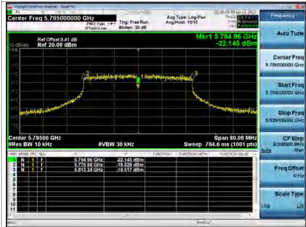
Freq. Stability 0C 120V n40 5795MHz Ant1 0 Minutes
