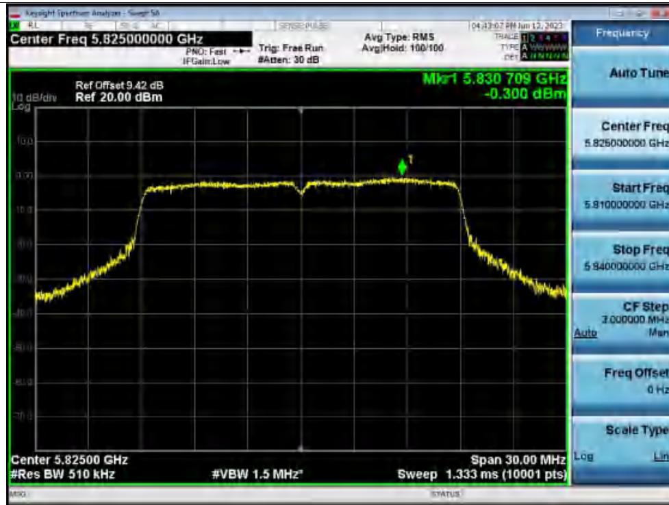
PSD NVNT n20 5825MHz Ant1
