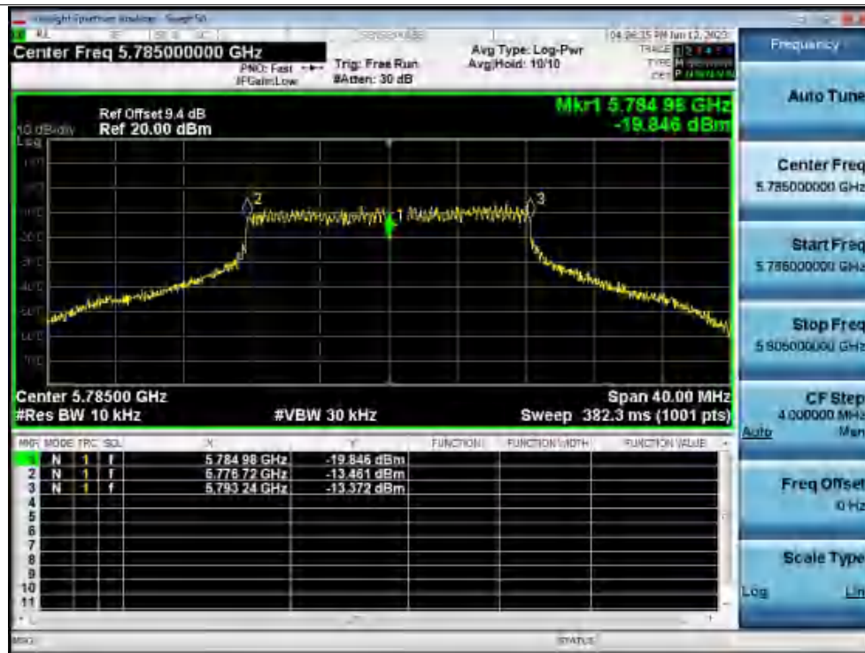
Freq. Stability 0C 120V a 5785MHz Ant1 0 Minutes
