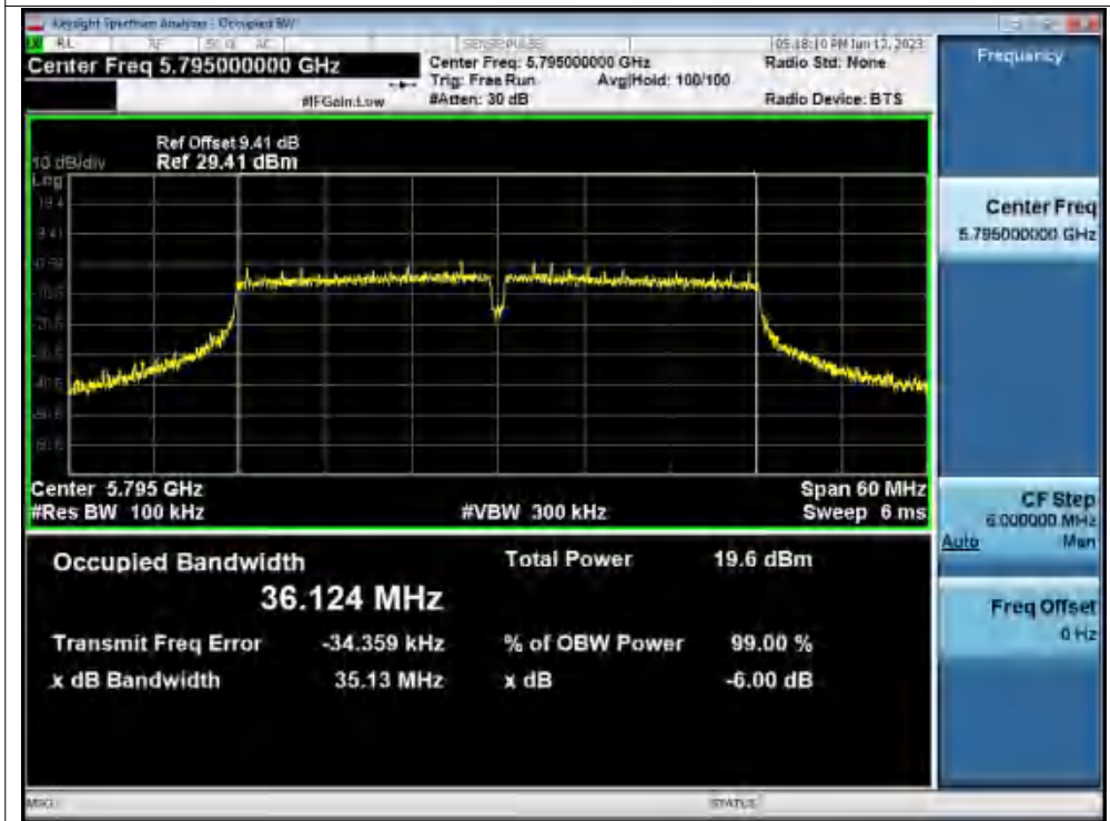
-6dB Bandwidth NVNT ac40 5795MHz Ant1
