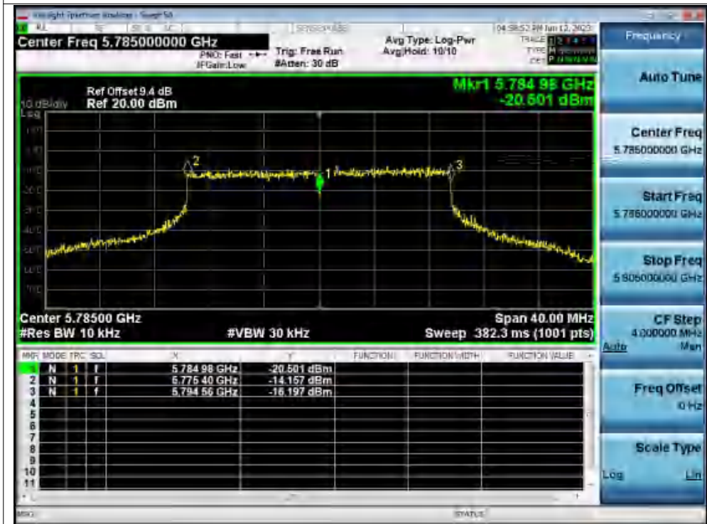
Freq. Stability 0C 120V ax20 5785MHz Ant1 0 Minutes
