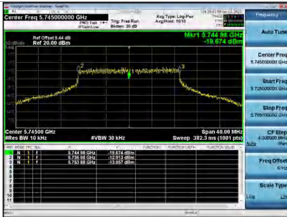
Freq. Stability 30C 120V n20 5745MHz Ant1 0 Minutes
