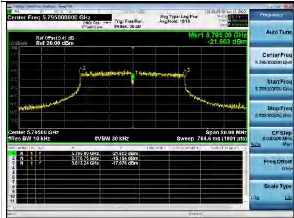
Freq. Stability 50C 120V n40 5795MHz Ant1 0 Minutes
