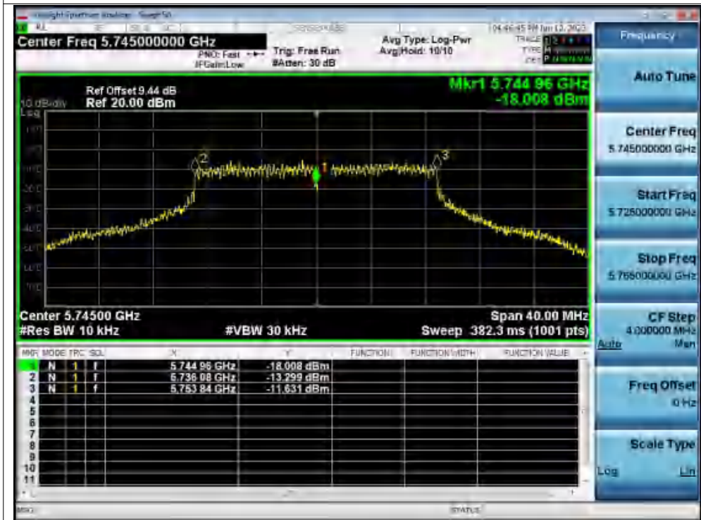
Freq. Stability -20C 120V ac20 5745MHz Ant1 0 Minutes
