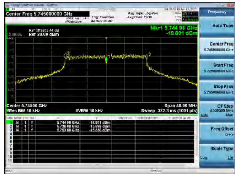
Freq. Stability 30C 120V n20 5745MHz Ant1 0 Minutes
