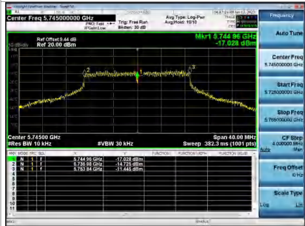
Freq. Stability 30C 120V ac20 5745MHz Ant1 0 Minutes
