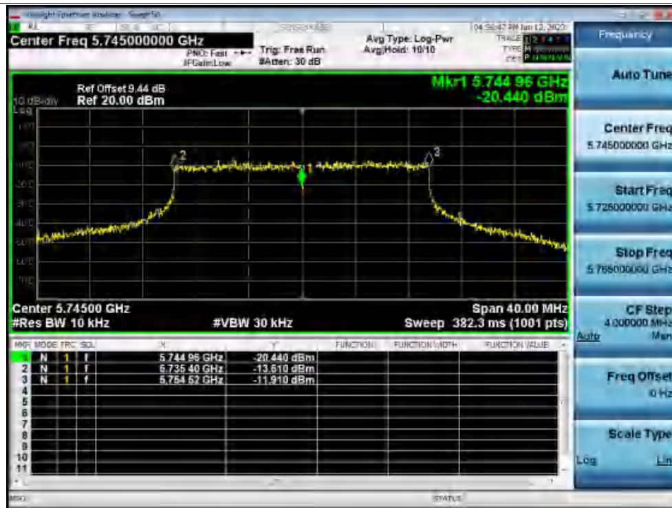
Freq. Stability 50C 120V ax20 5745MHz Ant1 0 Minutes
