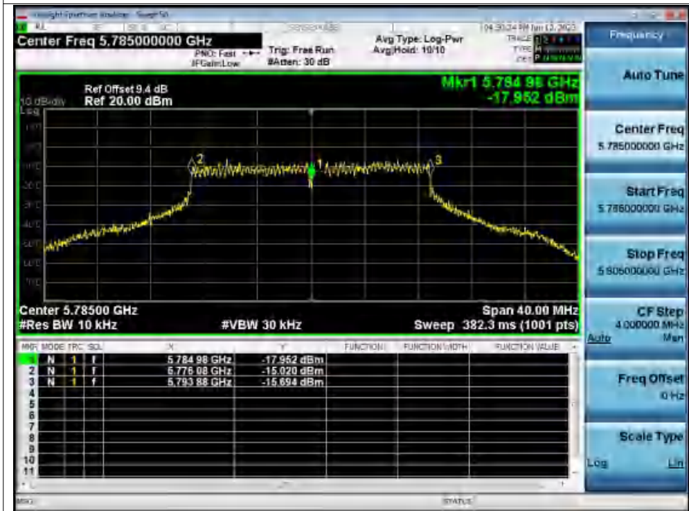
Freq. Stability 30C 120V ac20 5785MHz Ant1 0 Minutes
