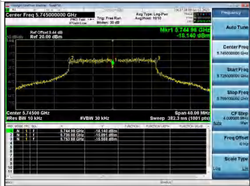
Freq. Stability 50C 120V ac20 5745MHz Ant1 0 Minutes
