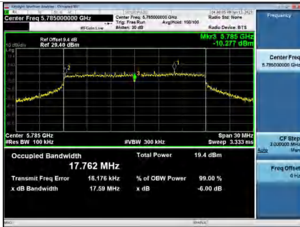
-6dB Bandwidth NVNT n20 5825MHz Ant1
