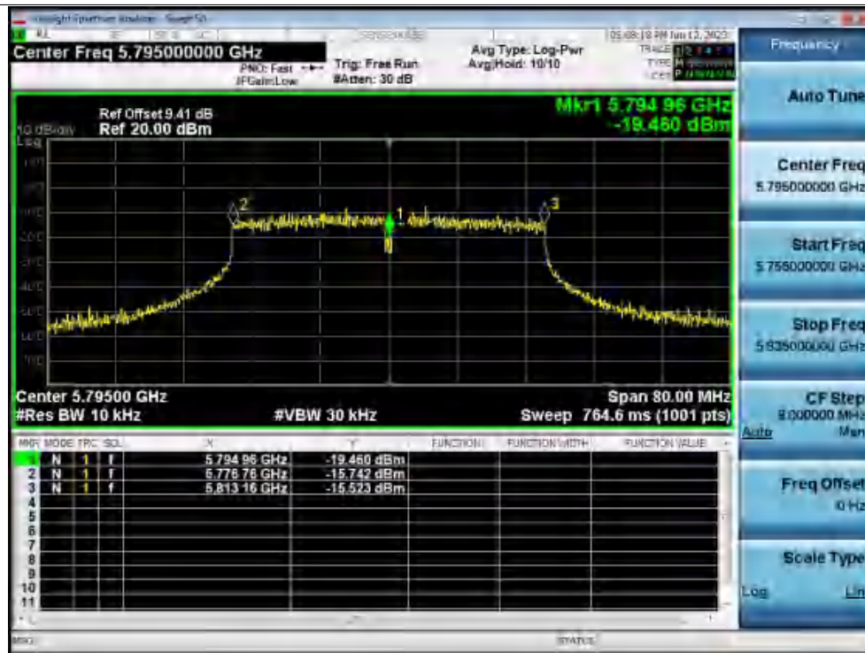
Freq. Stability 30C 120V n40 5795MHz Ant1 0 Minutes
