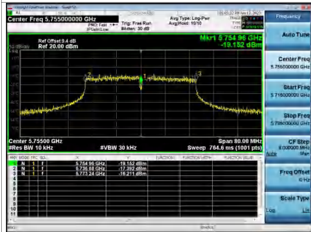
Freq. Stability 30C 120V n40 5755MHz Ant1 0 Minutes
