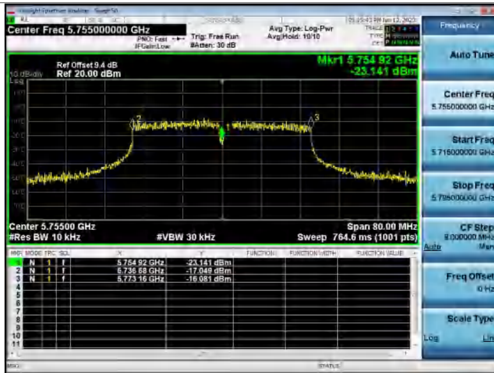
Freq. Stability 0C 120V ac40 5755MHz Ant1 0 Minutes
