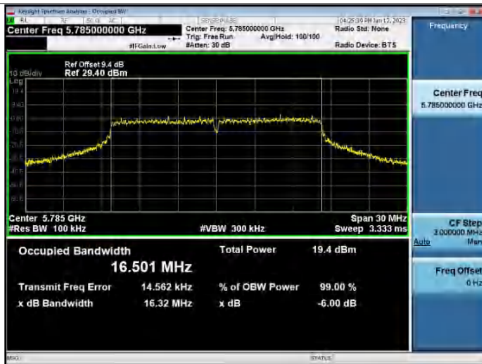
-6dB Bandwidth NVNT a 5785MHz Ant1
