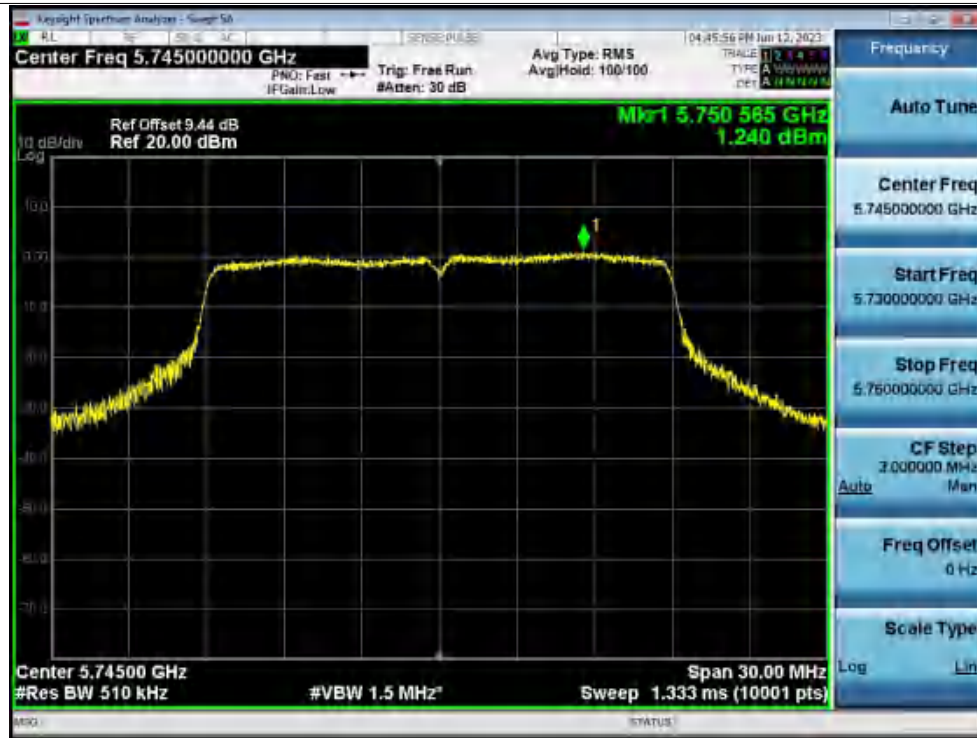
PSD NVNT ac20 5785MHz Ant1
