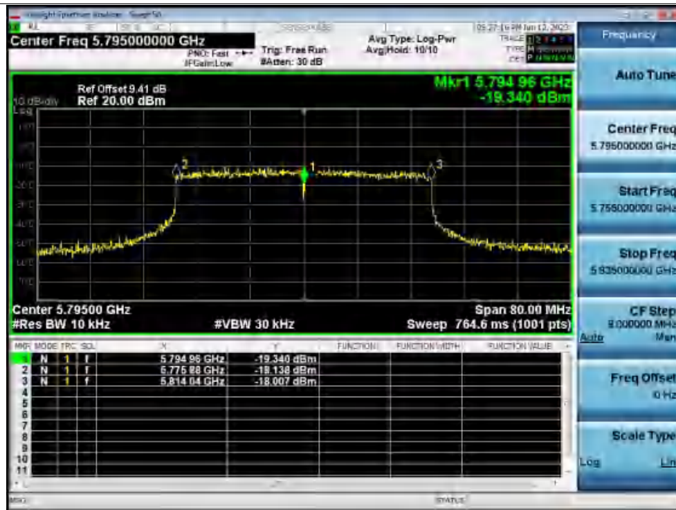
Freq. Stability 30C 120V ax40 5795MHz Ant1 0 Minutes
