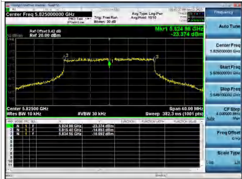
Freq. Stability 0C 120V ax20 5825MHz Ant1 0 Minutes
