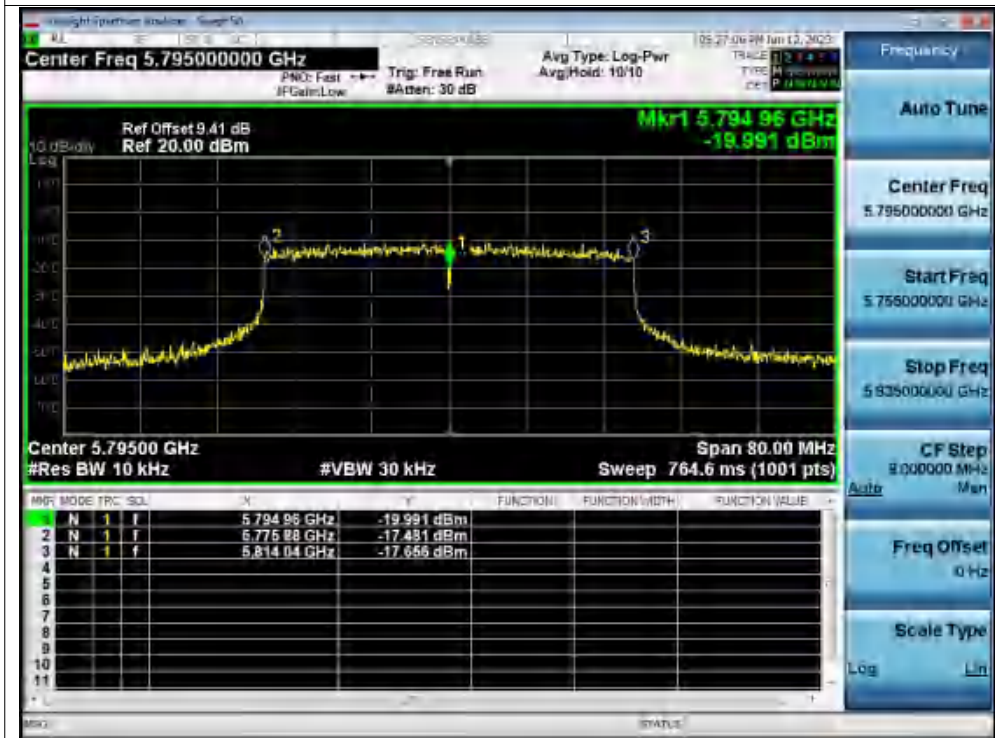
Freq. Stability 0C 120V ax40 5795MHz Ant1 0 Minutes
