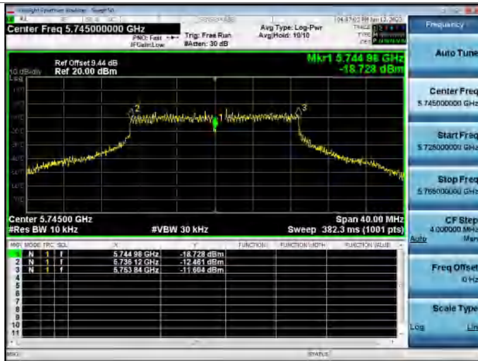
Freq. Stability 30C 120V ac20 5745MHz Ant1 0 Minutes
