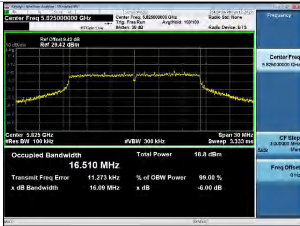
-6dB Bandwidth NVNT n20 5745MHz Ant1
