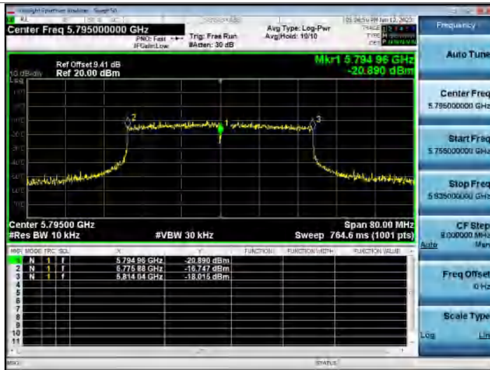
Freq. Stability 0C 120V ax40 5795MHz Ant1 0 Minutes
