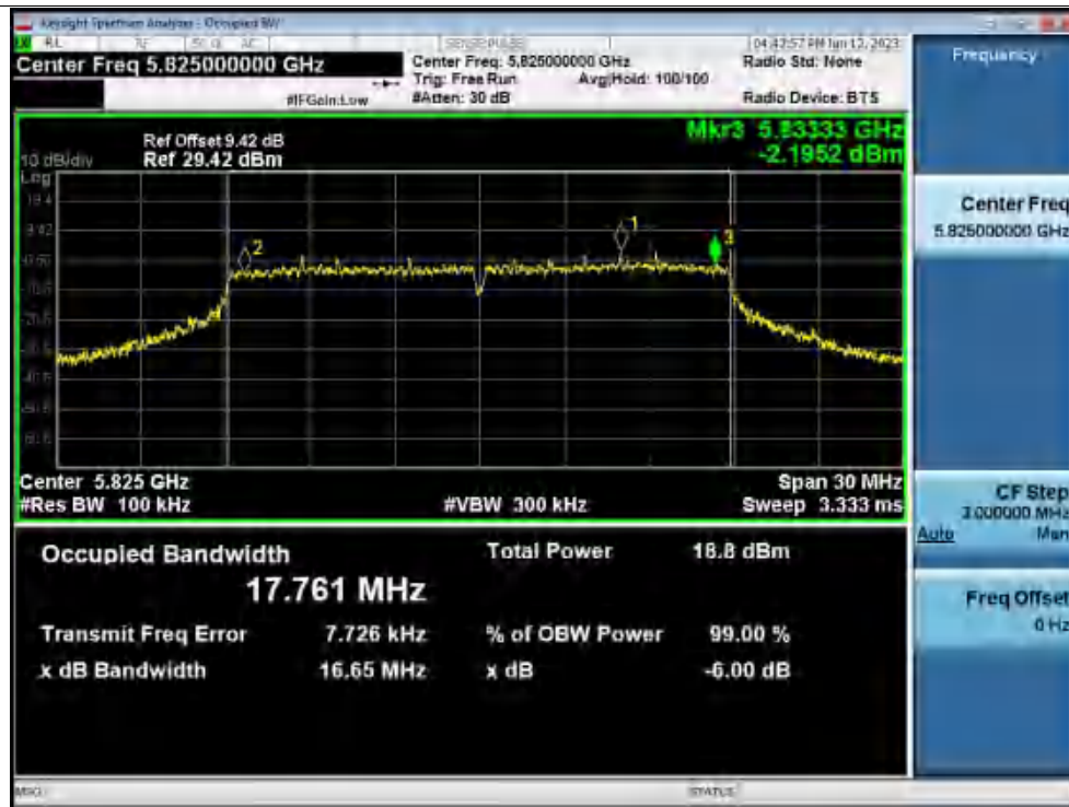
-6dB Bandwidth NVNT n20 5825MHz Ant1
