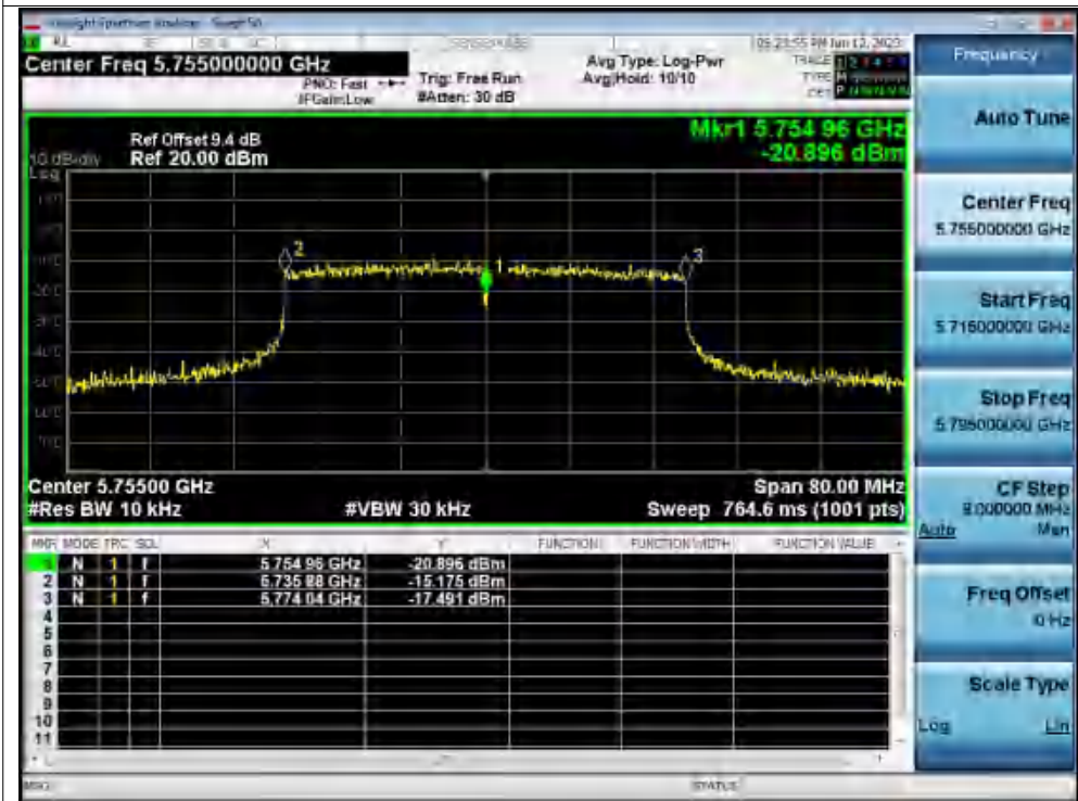
Freq. Stability 30C 120V ax40 5755MHz Ant1 0 Minutes
