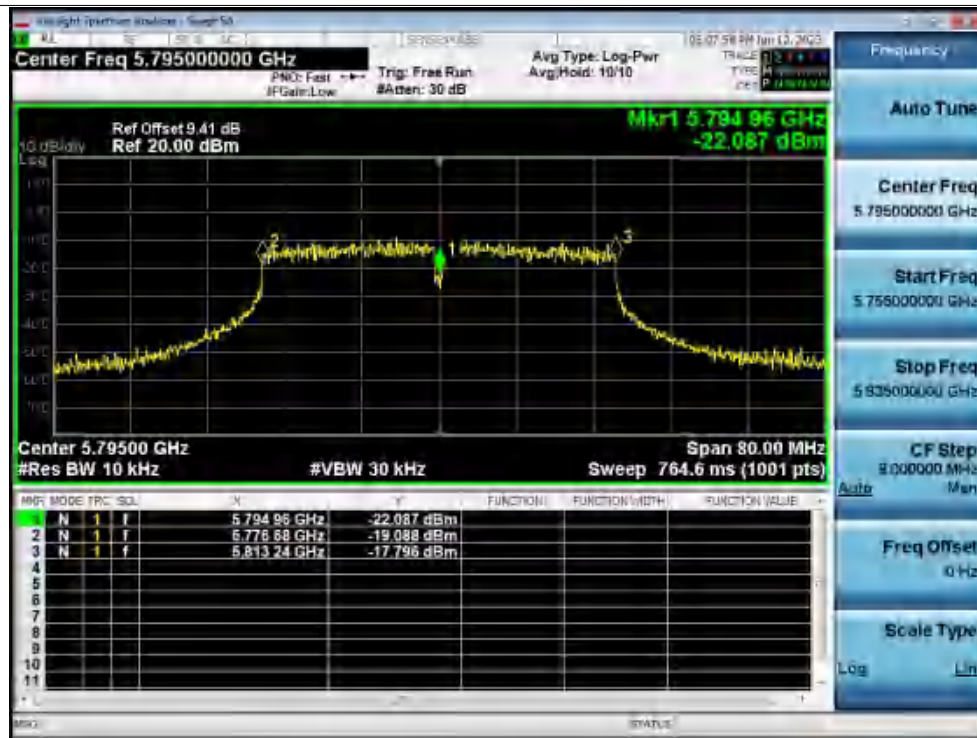
Freq. Stability 0C 120V n40 5795MHz Ant1 0 Minutes
