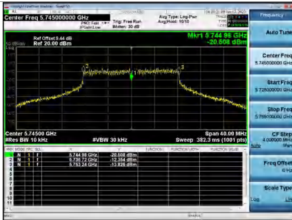
Freq. Stability 50C 120V a 5745MHz Ant1 0 Minutes
