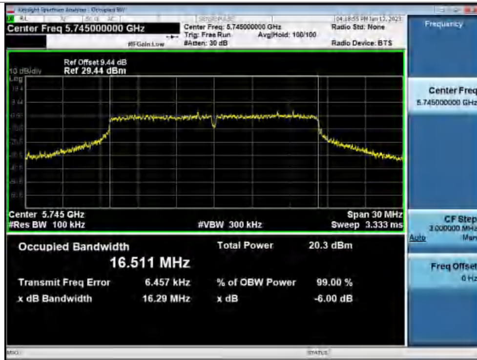
-6dB Bandwidth NVNT a 5785MHz Ant1
