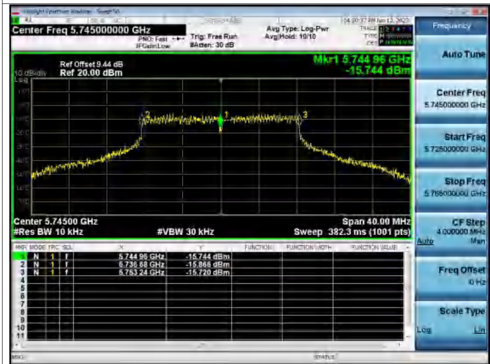
Freq. Stability 50C 120V a 5745MHz Ant1 0 Minutes
