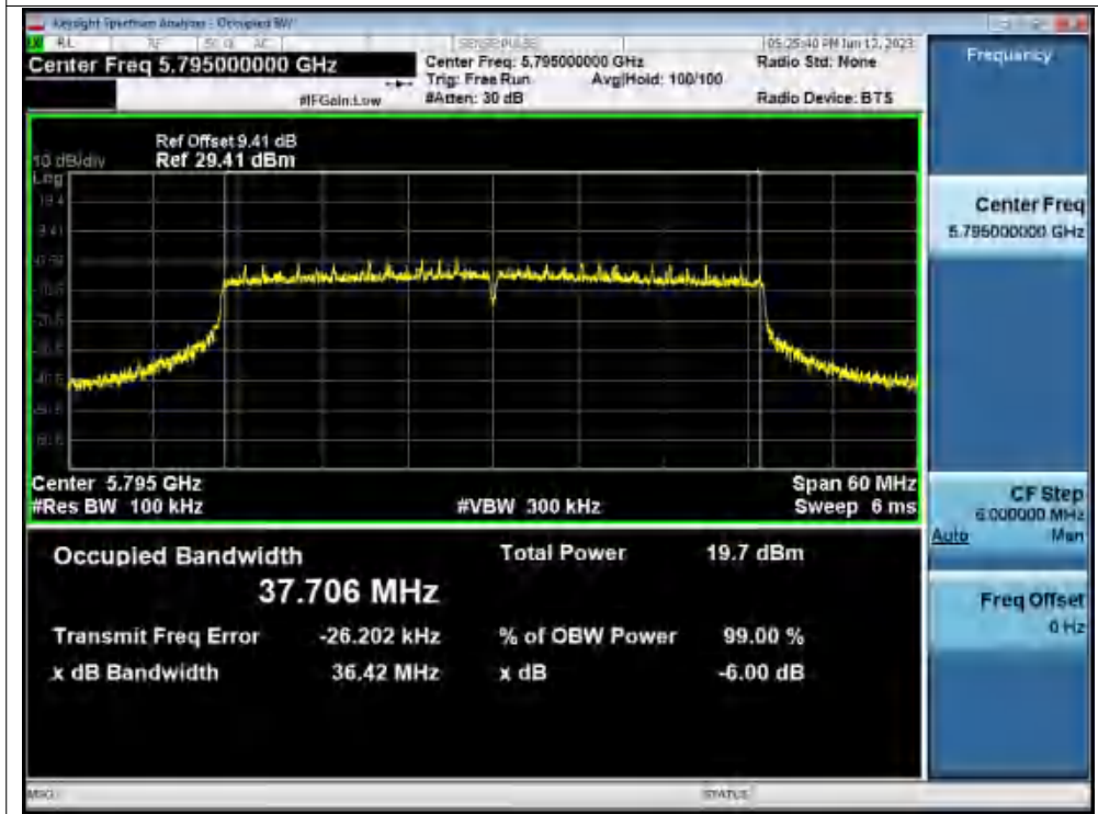
-6dB Bandwidth NVNT ax40 5795MHz Ant1
