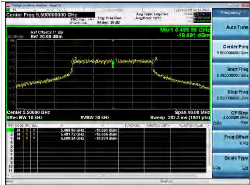
Freq. Stability 30C 120V a 5500MHz Ant1 0 Minutes
