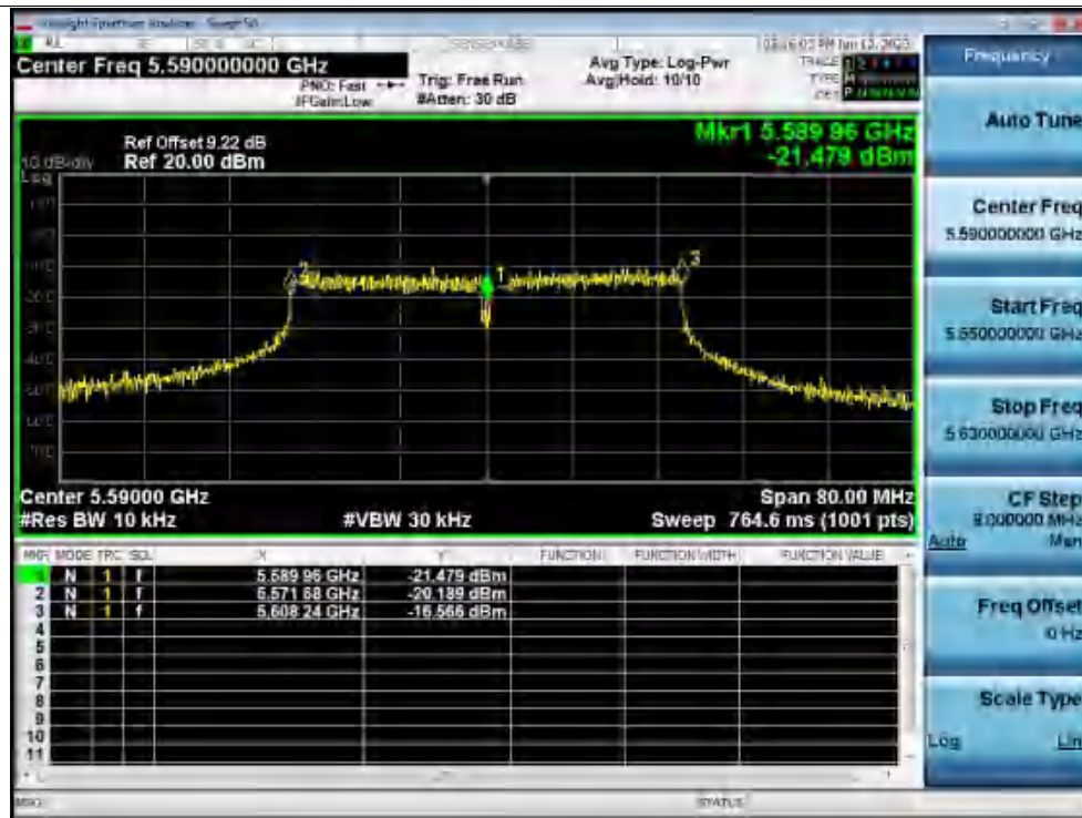
Freq. Stability 50C 120V n40 5590MHz Ant1 0 Minutes
