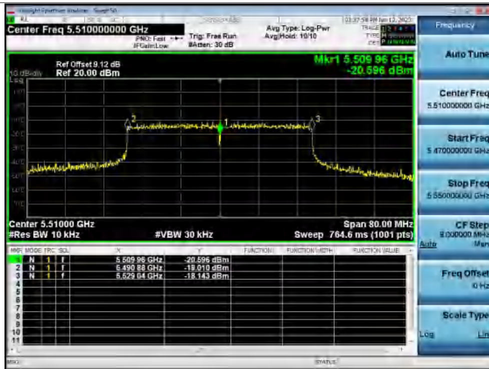
Freq. Stability 30C 120V ax40 5510MHz Ant1 0 Minutes
