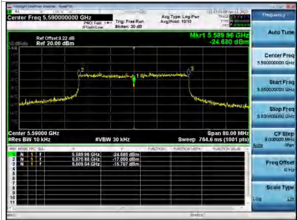
Freq. Stability 20C 120V ax40 5590MHz Ant1 0 Minutes
