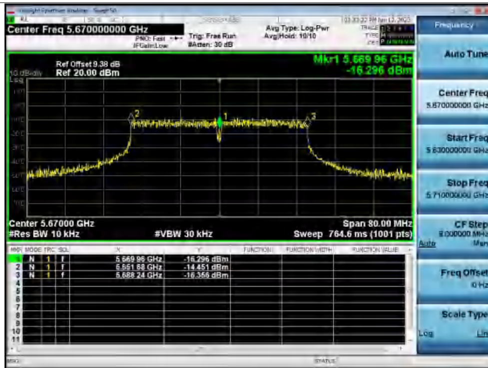
Freq. Stability -20C 120V ac40 5670MHz Ant1 0 Minutes
