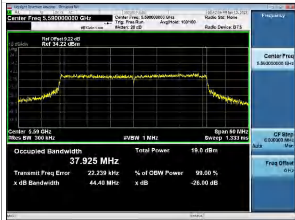
-26dB Bandwidth NVNT ax40 5590MHz Ant1
