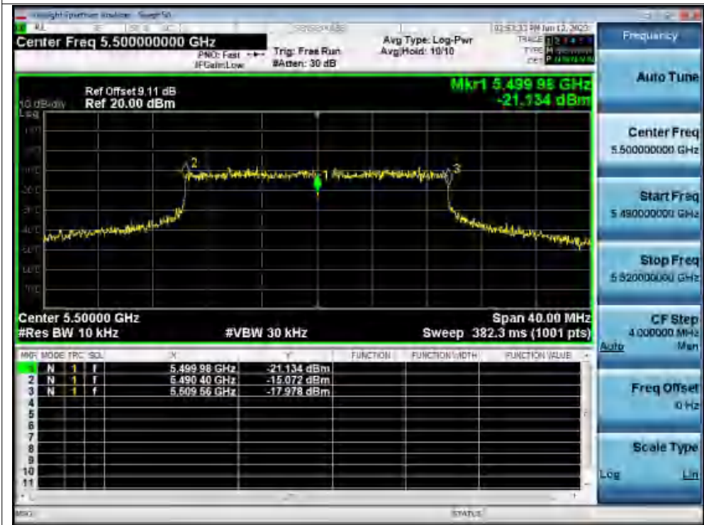
Freq. Stability 30C 120V ax20 5500MHz Ant1 0 Minutes
