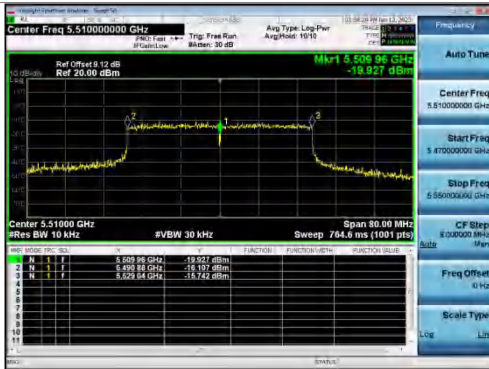
Freq. Stability 50C 120V ax40 5510MHz Ant1 0 Minutes
