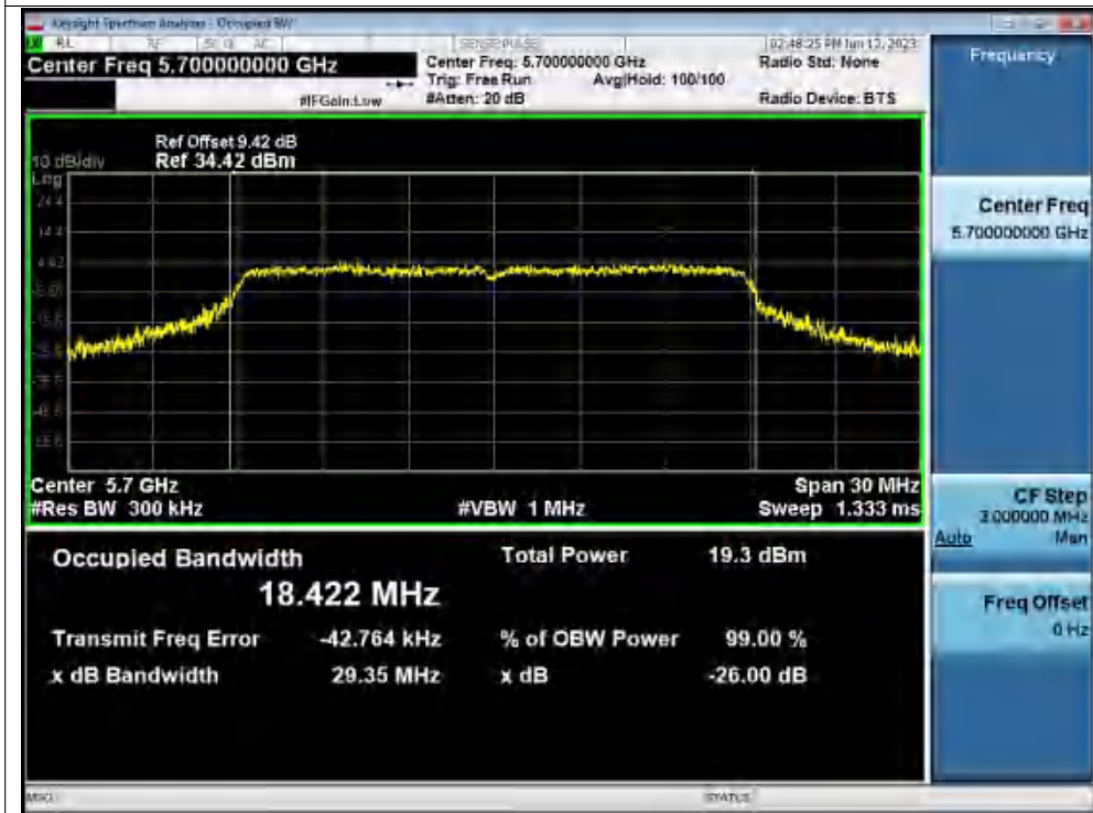
-26dB Bandwidth NVNT ac40 5510MHz Ant1
