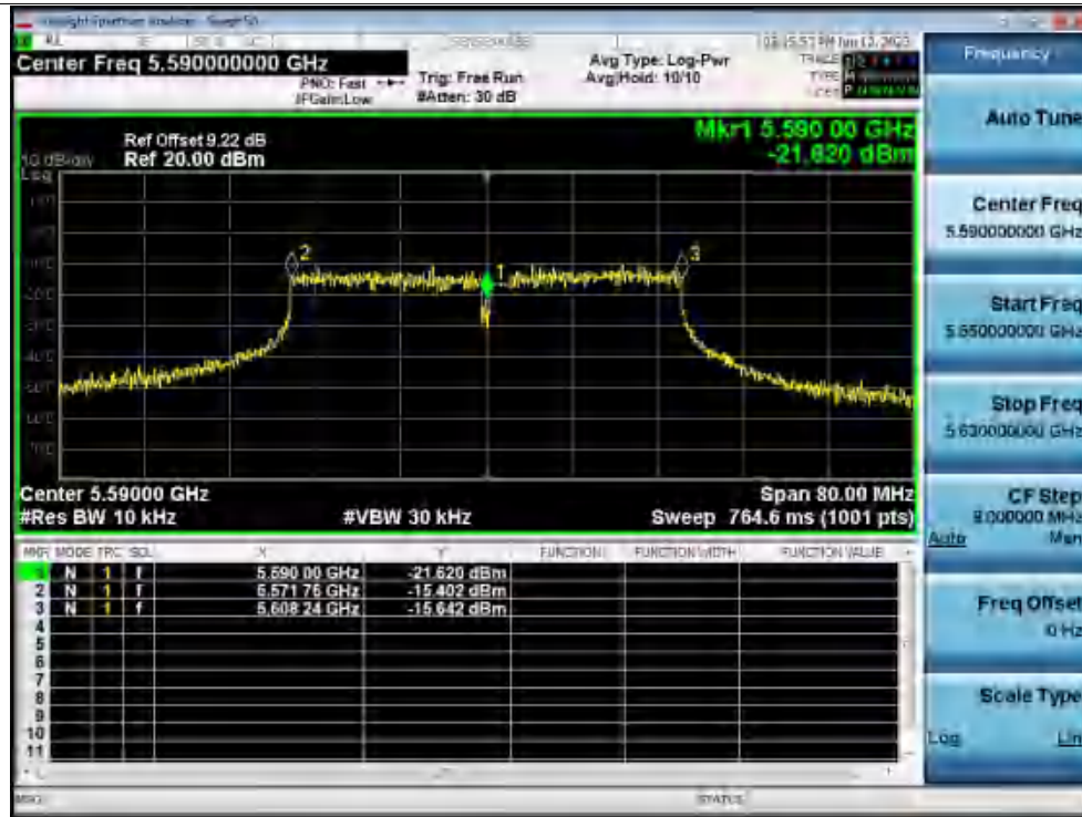
Freq. Stability 50C 120V n40 5590MHz Ant1 0 Minutes
