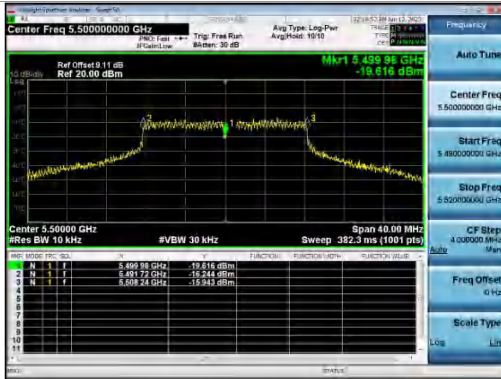
Freq. Stability -20C 120V a 5500MHz Ant1 0 Minutes
