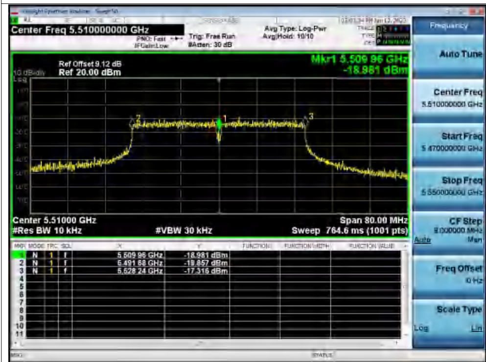
Freq. Stability 0C 120V n40 5510MHz Ant1 0 Minutes
