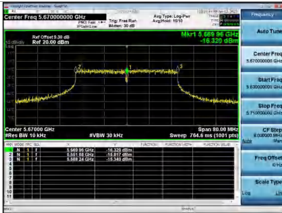
Freq. Stability 30C 120V n40 5670MHz Ant1 0 Minutes
