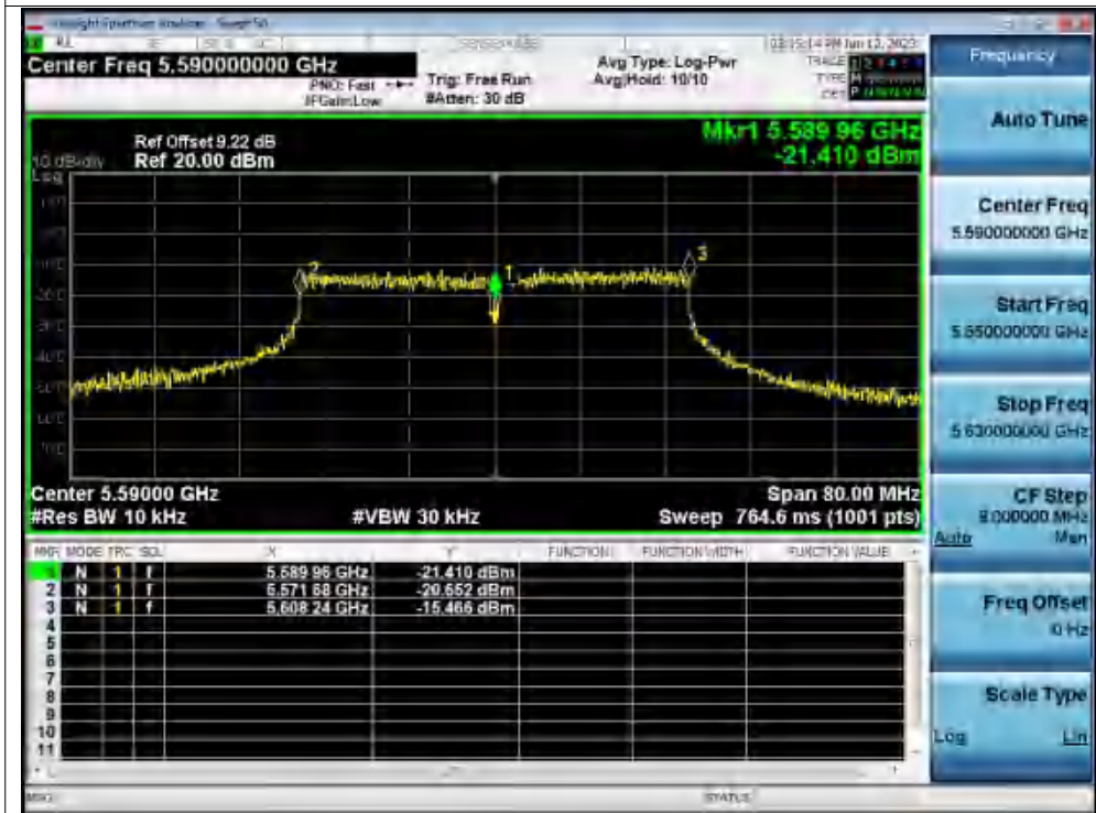
Freq. Stability 0C 120V n40 5590MHz Ant1 0 Minutes
