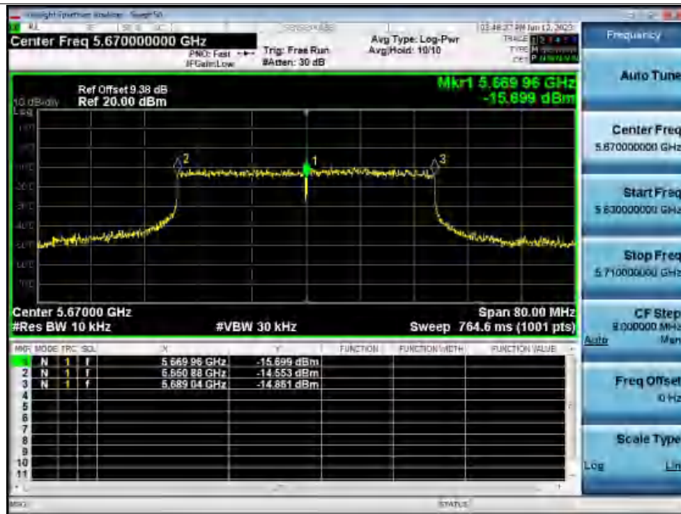
Freq. Stability 50C 120V ax40 5670MHz Ant1 0 Minutes
