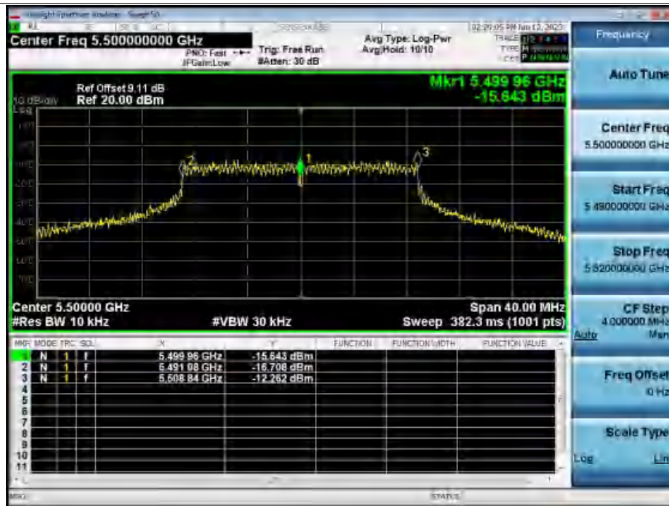
Freq. Stability 0C 120V n20 5500MHz Ant1 0 Minutes
