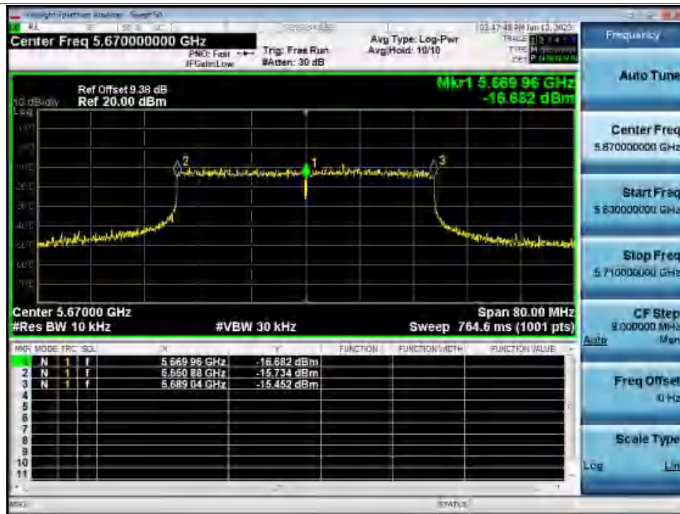
Freq. Stability 30C 120V ax40 5670MHz Ant1 0 Minutes
