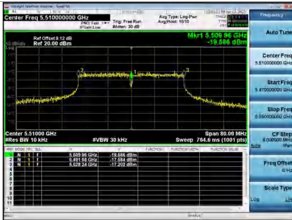
Freq. Stability 0C 120V n40 5510MHz Ant1 0 Minutes
