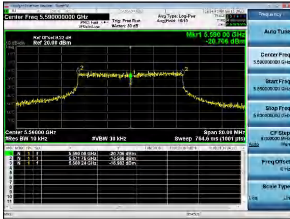
Freq. Stability -20C 120V n40 5590MHz Ant1 0 Minutes
