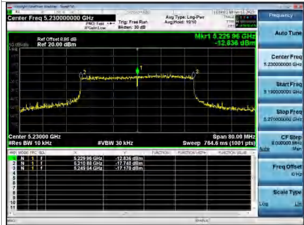
Freq. Stability -20C 120V ax40 5230MHz Ant1 0 Minutes
