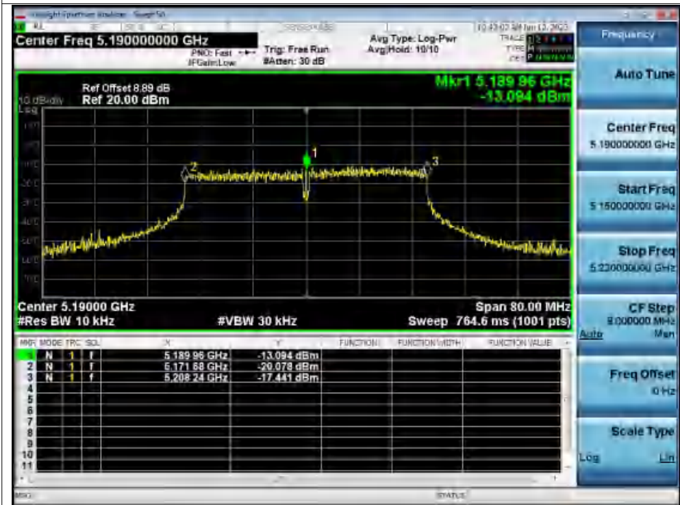
Freq. Stability -20C 120V n40 5190MHz Ant1 0 Minutes
