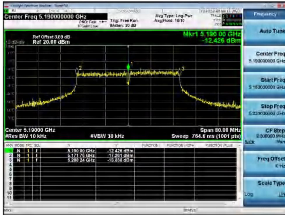
Freq. Stability -20C 120V n40 5190MHz Ant1 0 Minutes
