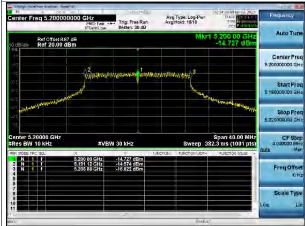
Freq. Stability 30C 120V ac20 5200MHz Ant1 0 Minutes
