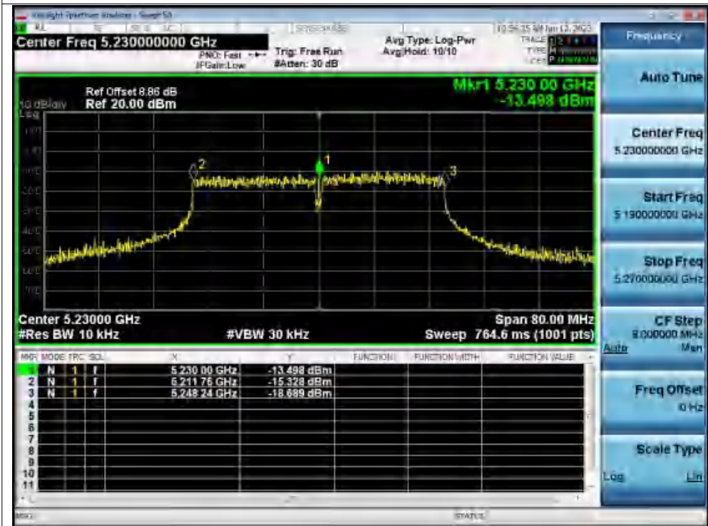
Freq. Stability 50C 120V ac40 5230MHz Ant1 0 Minutes
