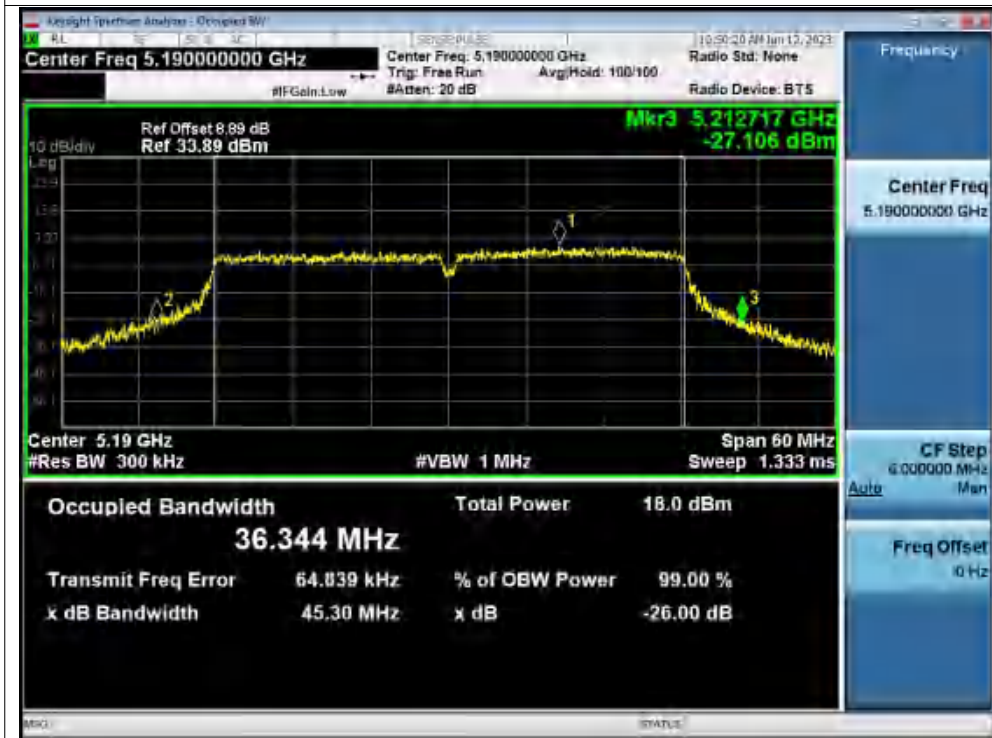
-26dB Bandwidth NVNT ac40 5190MHz Ant1
