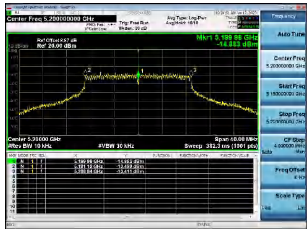
Freq. Stability 50C 120V ac20 5200MHz Ant1 0 Minutes
