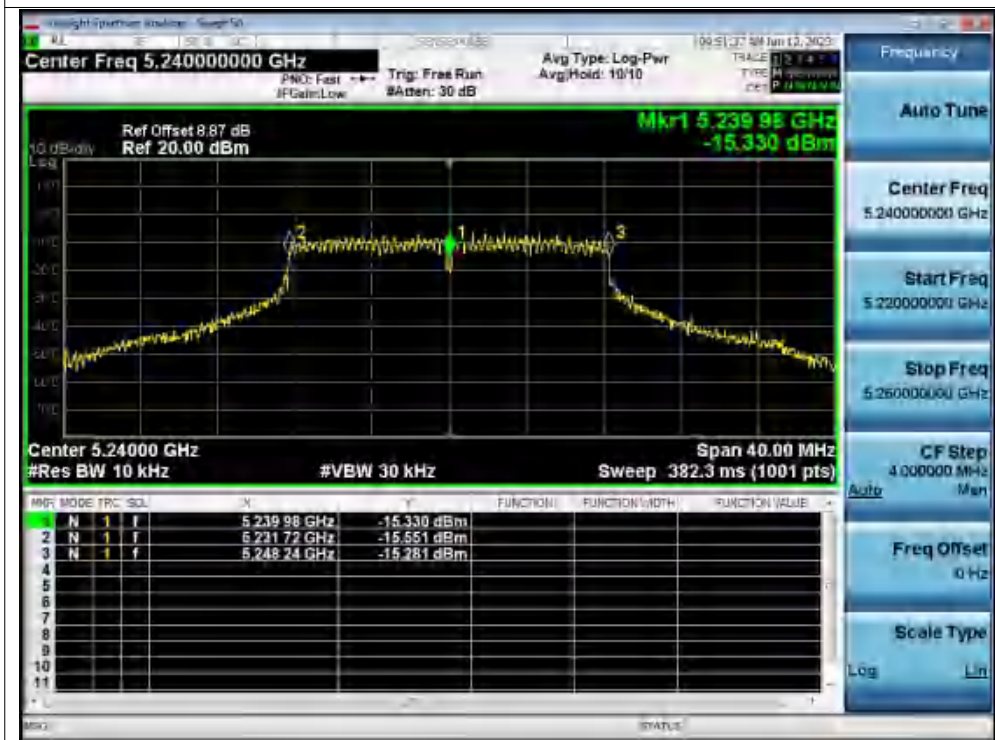
Freq. Stability 50C 120V a 5240MHz Ant1 0 Minutes
