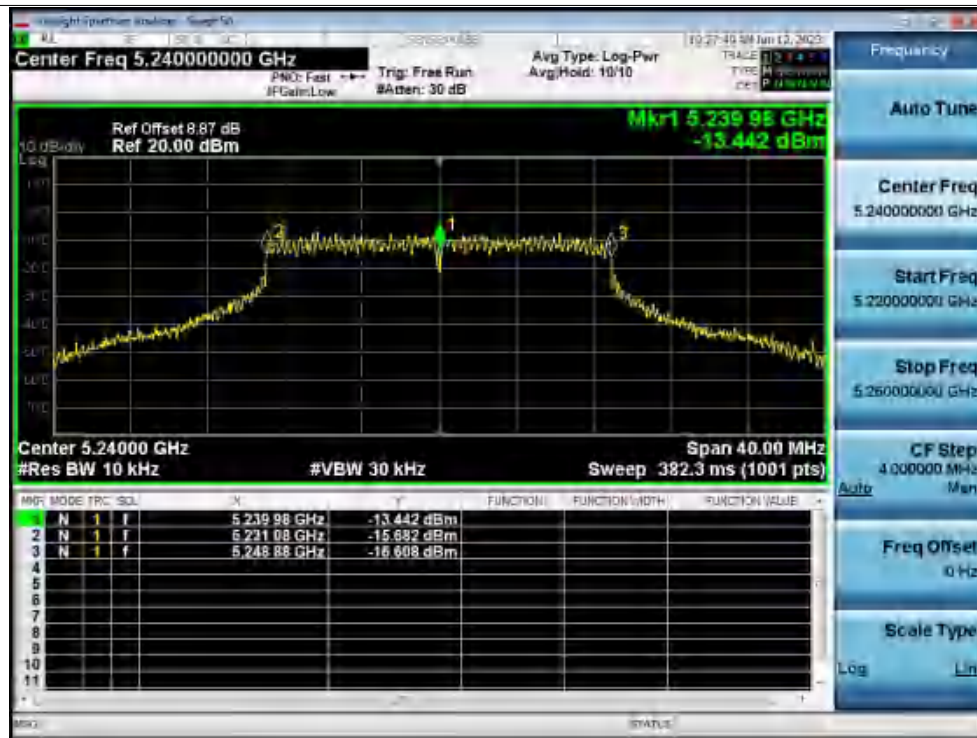
Freq. Stability 0C 120V ac20 5240MHz Ant1 0 Minutes
