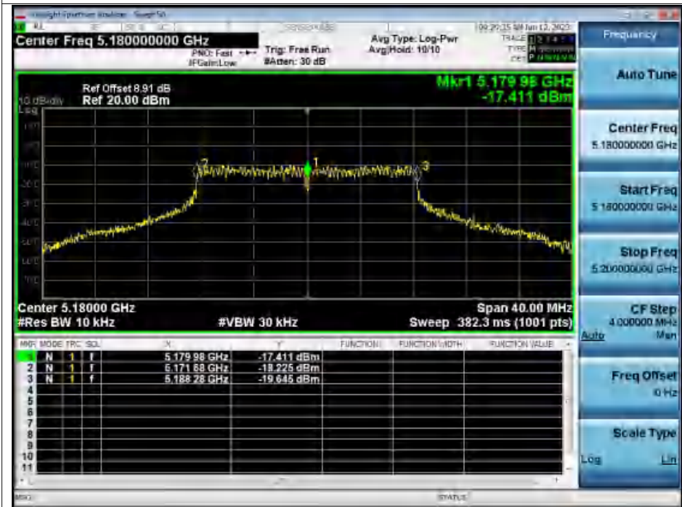
Freq. Stability -20C 120V a 5180MHz Ant1 0 Minutes
