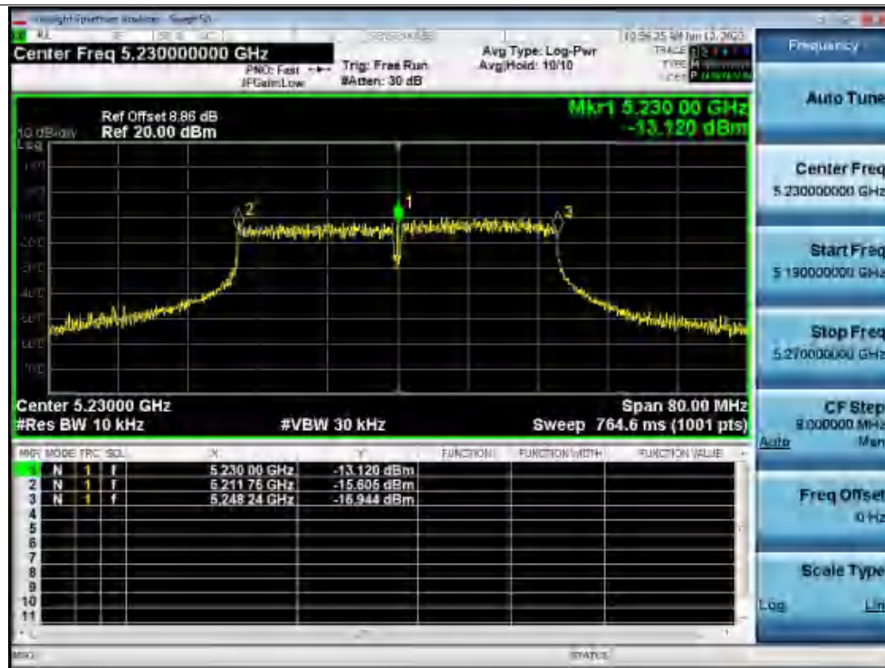
Freq. Stability 50C 120V ac40 5230MHz Ant1 0 Minutes
