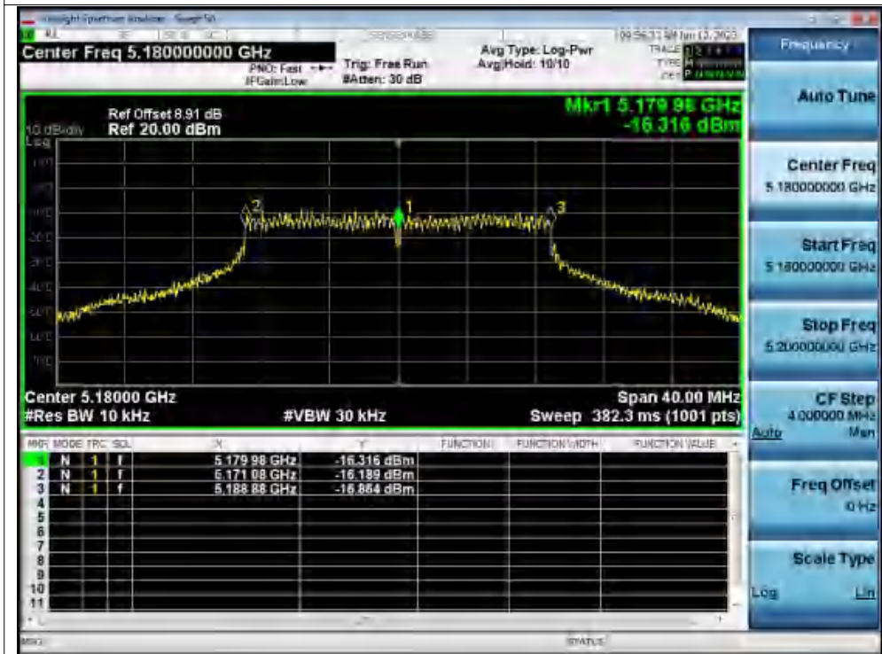
Freq. Stability 0C 120V n20 5180MHz Ant1 0 Minutes
