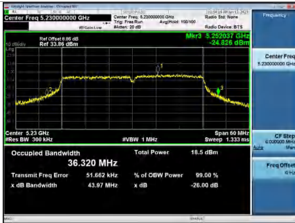
-26dB Bandwidth NVNT ax20 5180MHz Ant1
