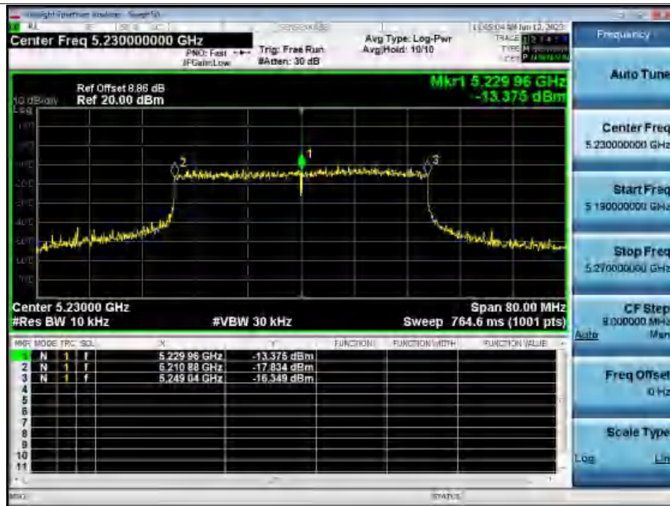
Freq. Stability 50C 120V ax40 5230MHz Ant1 0 Minutes
