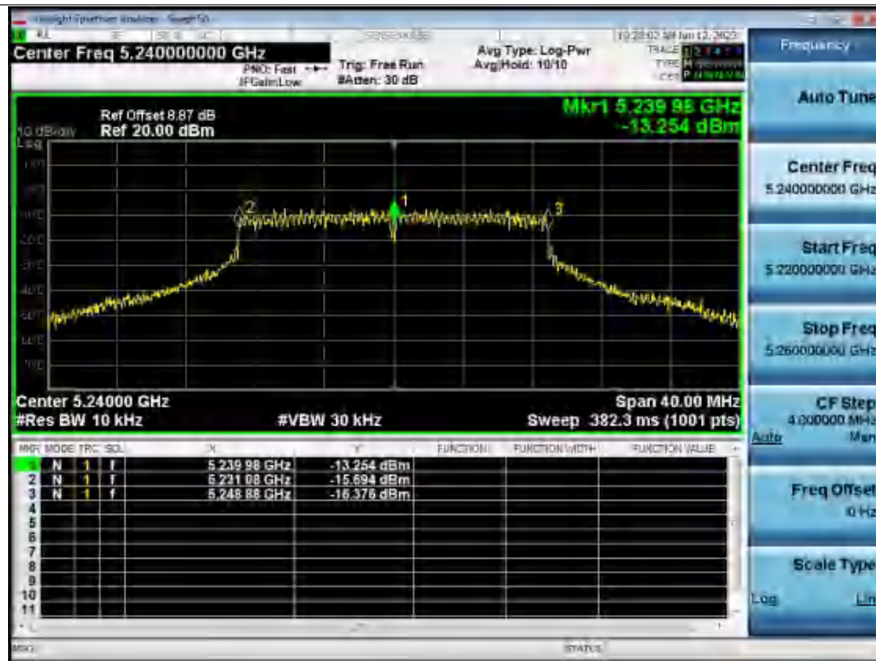
Freq. Stability 30C 120V ac20 5240MHz Ant1 0 Minutes
