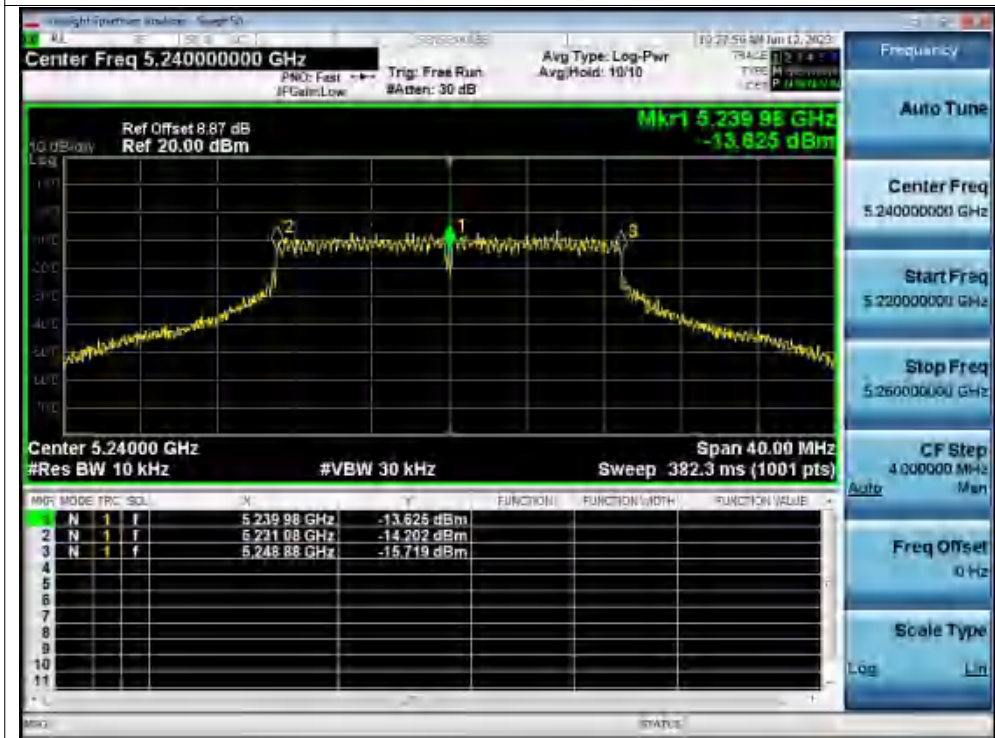
Freq. Stability 0C 120V ac20 5240MHz Ant1 0 Minutes
