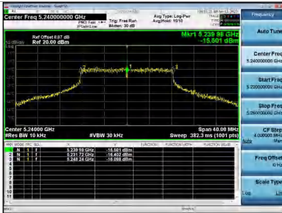
Freq. Stability 50C 120V a 5240MHz Ant1 0 Minutes
