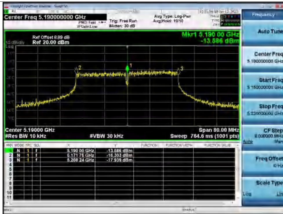
Freq. Stability 30C 120V ac40 5190MHz Ant1 0 Minutes
