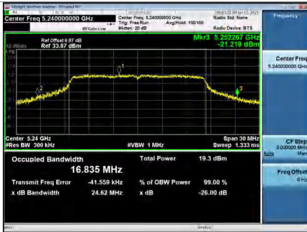
-26dB Bandwidth NVNT n20 5180MHz Ant1
