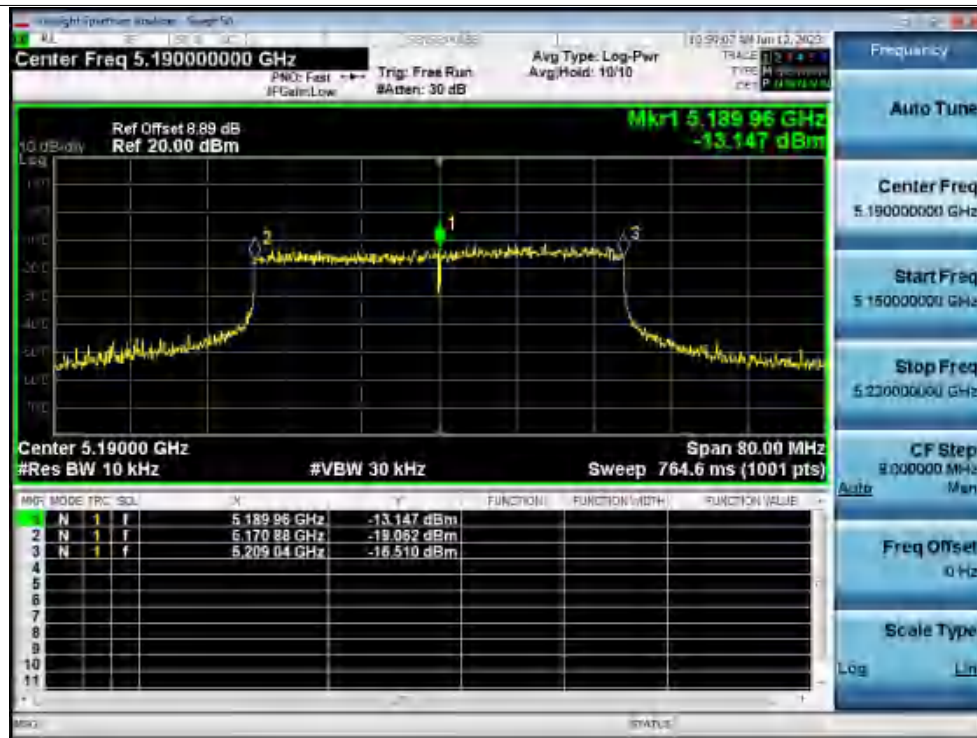
Freq. Stability -20C 120V ax40 5190MHz Ant1 0 Minutes
