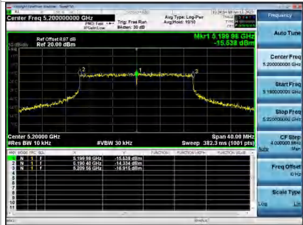
Freq. Stability 0C 120V ax20 5200MHz Ant1 0 Minutes
