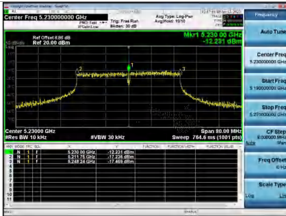
Freq. Stability 30C 120V n40 5230MHz Ant1 0 Minutes
