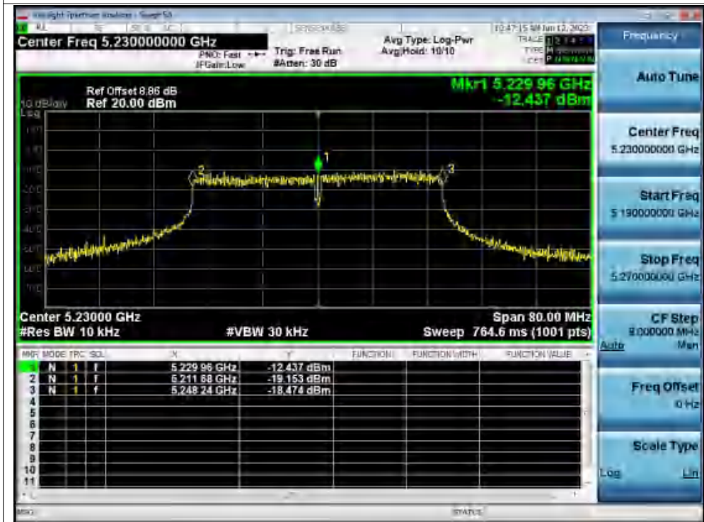
Freq. Stability -20C 120V n40 5230MHz Ant1 0 Minutes
