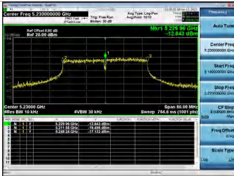
Freq. Stability 30C 120V ac40 5230MHz Ant1 0 Minutes
