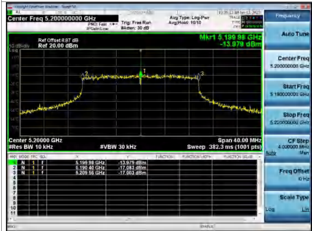
Freq. Stability 30C 120V ax20 5200MHz Ant1 0 Minutes
