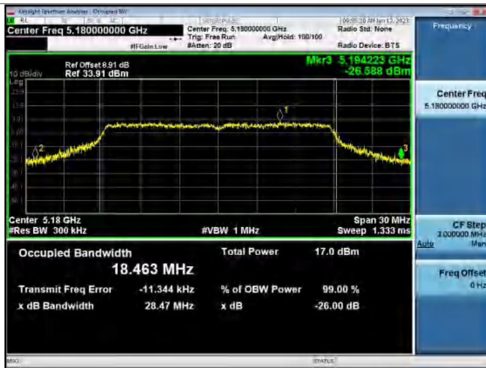
-26dB Bandwidth NVNT n20 5180MHz Ant1
