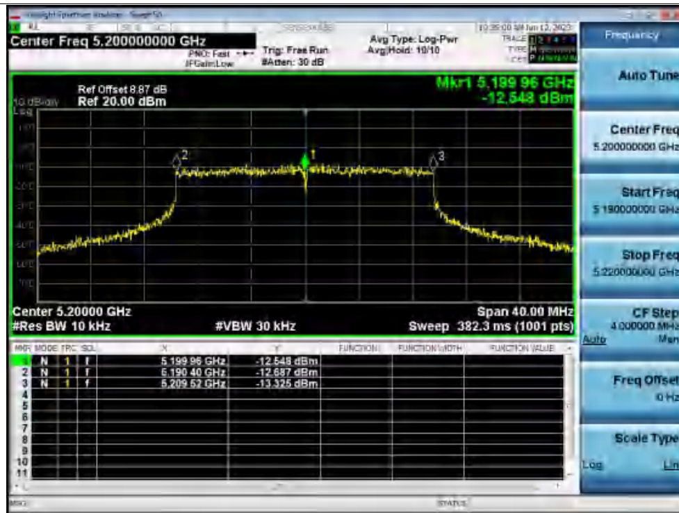
Freq. Stability 30C 120V ax20 5200MHz Ant1 0 Minutes
