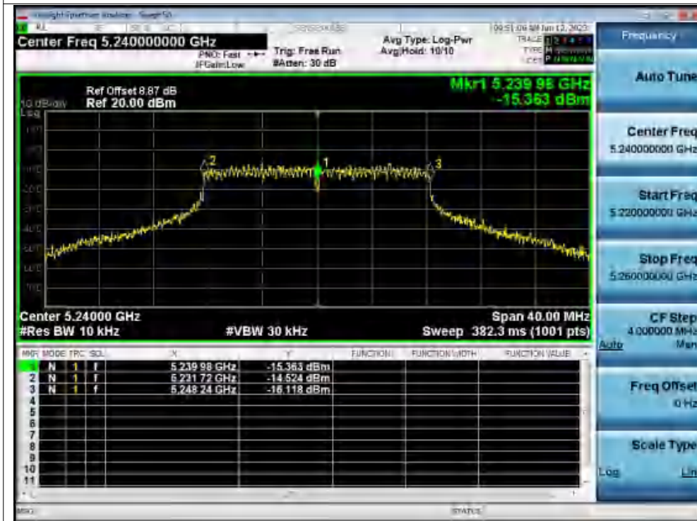
Freq. Stability 0C 120V a 5240MHz Ant1 0 Minutes
