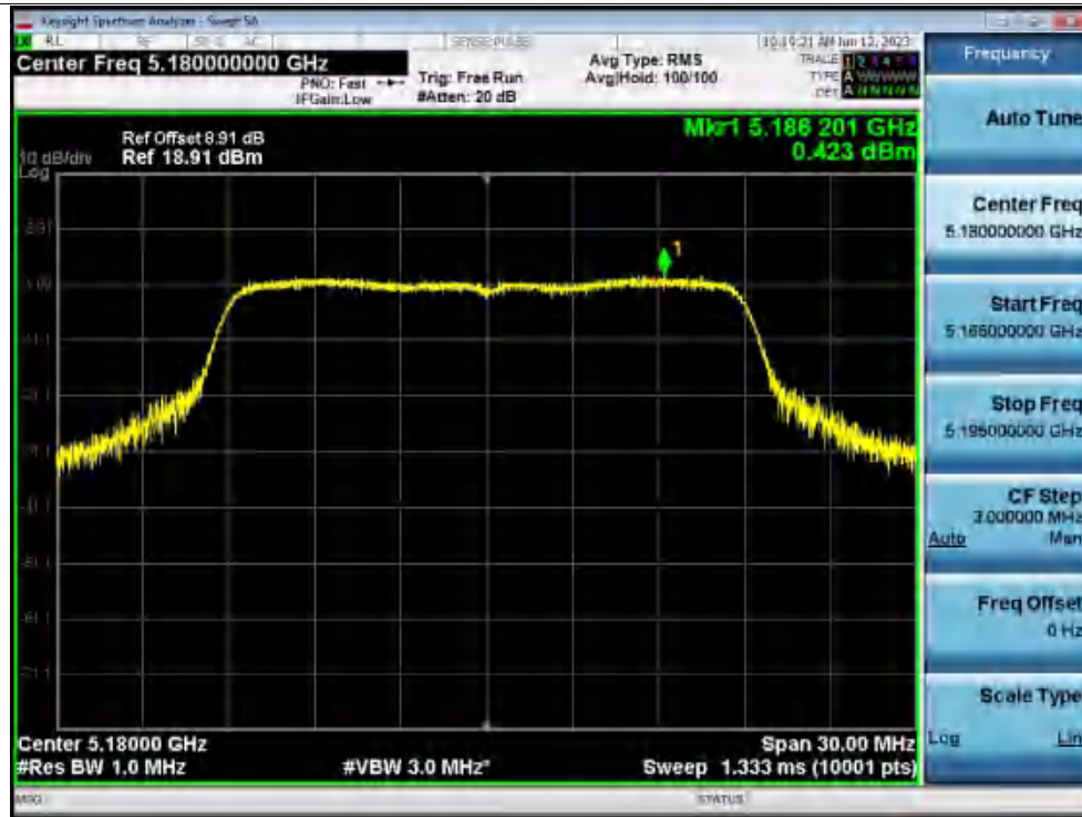
PSD NVNT ac20 5200MHz Ant1
