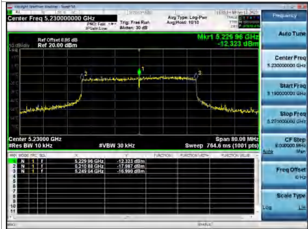
Freq. Stability 50C 120V ax40 5230MHz Ant1 0 Minutes
