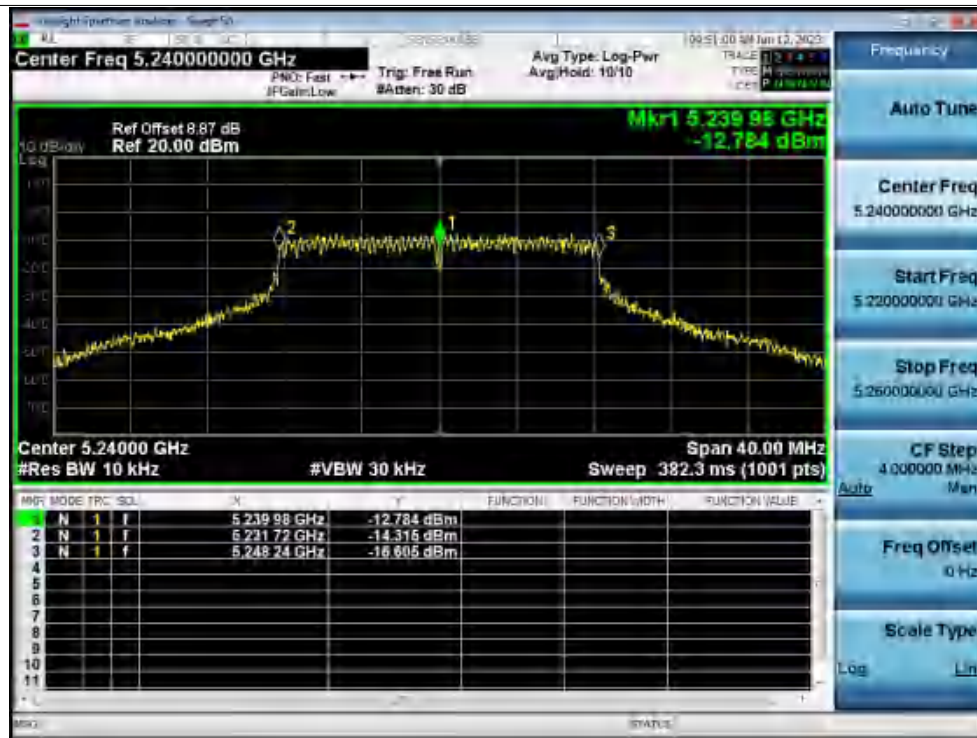
Freq. Stability 0C 120V a 5240MHz Ant1 0 Minutes
