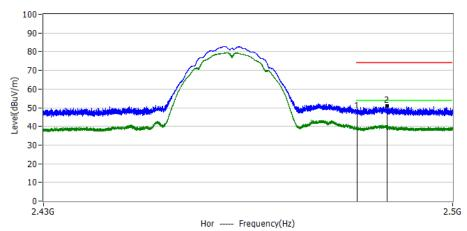
Frequency Reading Factor Level Limit Margin Polar No. Detector MHz dBuV dB/m dBuV/m dBuV/m dΒ 1\* 2483.5000 13.77 34.13 47.90 74.00 -26.10 PK Hor 2\* 2488.6000 16.62 34.14 50.76 74.00 -23.24 PΚ Hor
