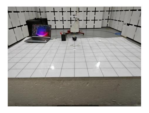
**Set-up for Radiated Spurious Emission, Above 1GHz**
