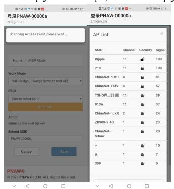
The A3. WIFI signal amplifier will automatically scan the surrounding WIFI signals, please select the WIFI signal that you want to connect (the following is only explained for example by connecting the 219 WIFI router). A password input interface will pop up, please enter the WIFI password for the router you want to relay amplification
