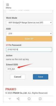
The A4. arrow is a modifiable area, and you can select the name of your device that you want to modify. Name is a combination of letters and numbers, and do not use non-ASIC characters. Because to optimize the system speed as possible, the device omitted support for complex characters.
