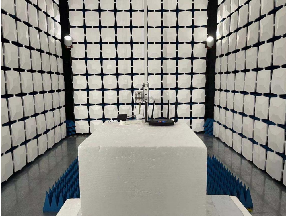
Above 1GHz for radiated emission test setup
