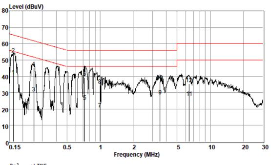
Test Mode: 03; Line: Live line; Modulation:802.11b; Bandwidth:20MHz; Channel:Low
