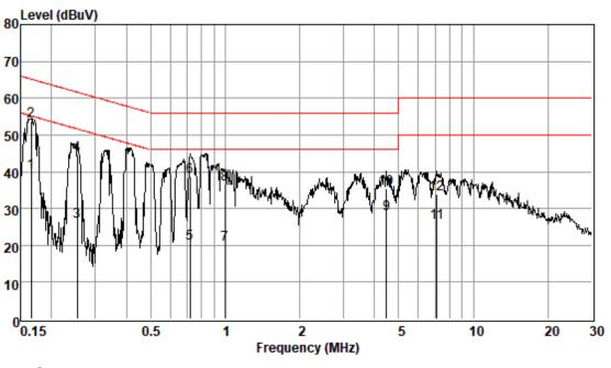
Test Mode: 03; Line: Neutral Line; Modulation:802.11b; Bandwidth:20MHz; Channel:Low
