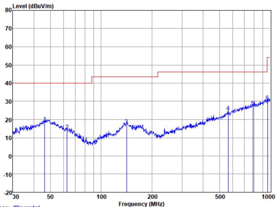
Test Mode: 3; Polarity: Vertical; Modulation:802.11b; Bandwidth:20MHz; Channel:Low
