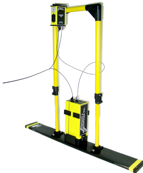
Figure 8: Close up of inter-changeable dipole antennas with full bistatic handle and electronics module attached. The fibre optics cables and beeper trigger are also shown.
