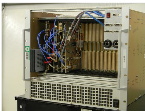
Figure 1. The FlexSAR-L VME chassis.
