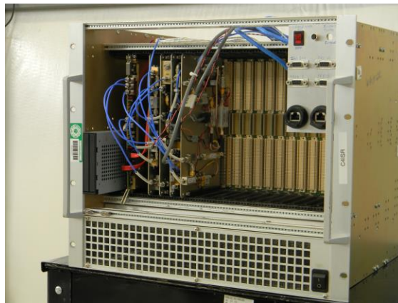
Figure 1. The FlexSAR-X VME chassis.
