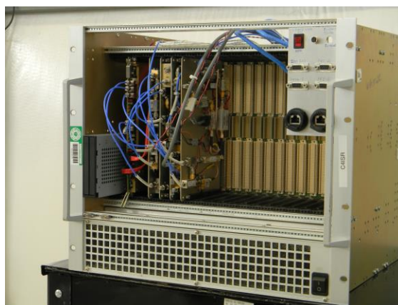
Figure 1. The FlexSAR-X VME chassis.
