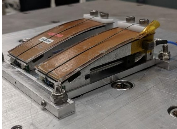
Fig 4. Experimental arrangement for bimorph release mechanism and vibration testing.
