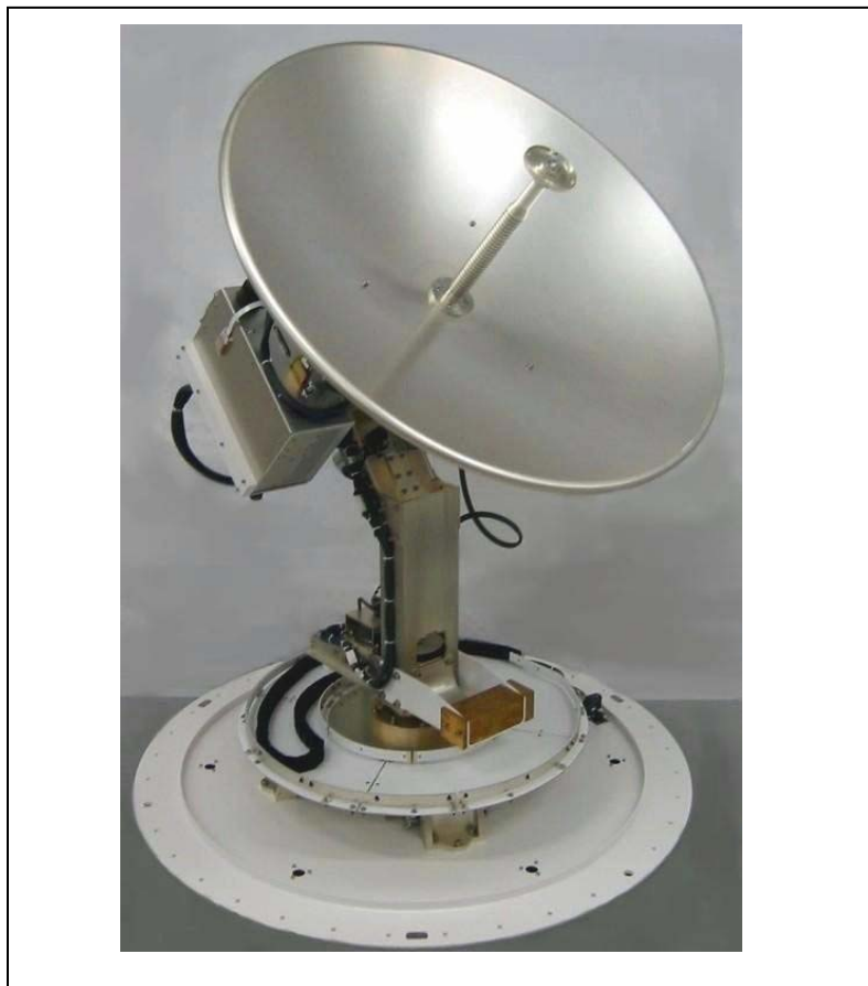
Figure 2. Illustration of a typical Melco 1.0 m antenna
