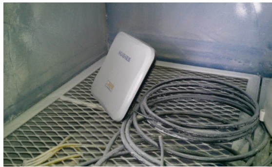
Picture of the Portable Antenna undergoing IP5X dust test
