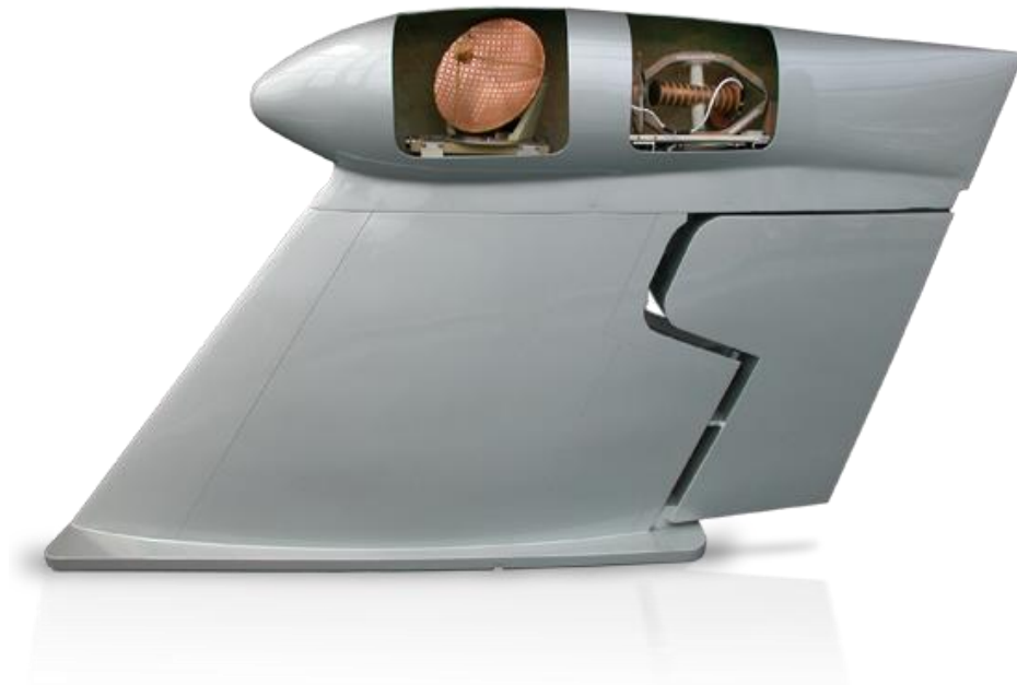
Figure 17: Typical tail mount for SatCom satellite system.
