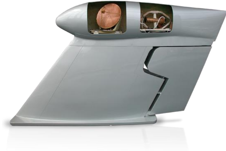
Figure 13: Typical tail mount for SatCom satellite system.
