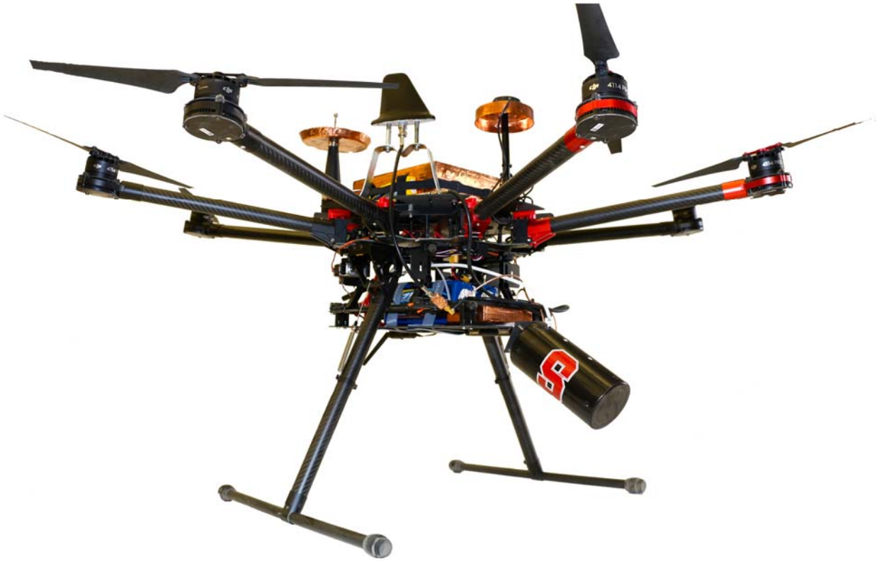
JAGER UAV based on DJI S1000. Hosts either of the two mobile antennas (RFD900+ and 3DR Radio) for telemetry. Wingspan is 1 m (1000 mm)
