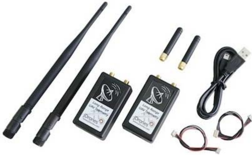
RFD900+ made by RFDesign (shorter antenna are for the mobile vehicle, antenna dimensions are 51mm long, 8mm diameter)
