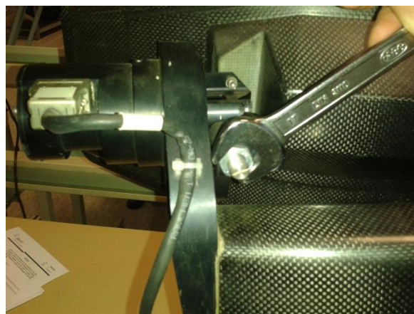
Figure 8 Mechanical stop releasing
