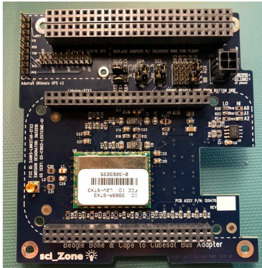
Figure 6: The LinkStar-STX3-PC104 Radio System.
