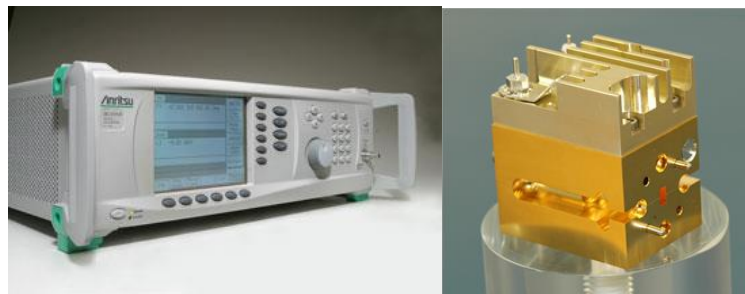
Figure 5 Left: Anritsu 67 GHz signal generator, Middle: Millitech AMC-10-RFHB0 75 to 110 GHz active multiplier needed to generate signals from 75 to 110 GHz (uses an input of 12.5 to 18.33 GHz 6 times multiplication).
