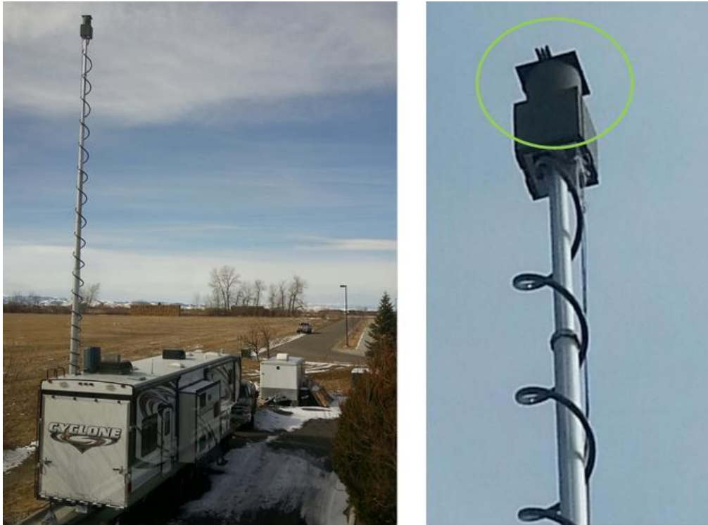
Figure 2 Antenna on top of mast on RV and S2 hardware in the garage of the RV. Doing direction finding, see truck in the distance down the road, which is transmitting with FCC approval across a wide band.
