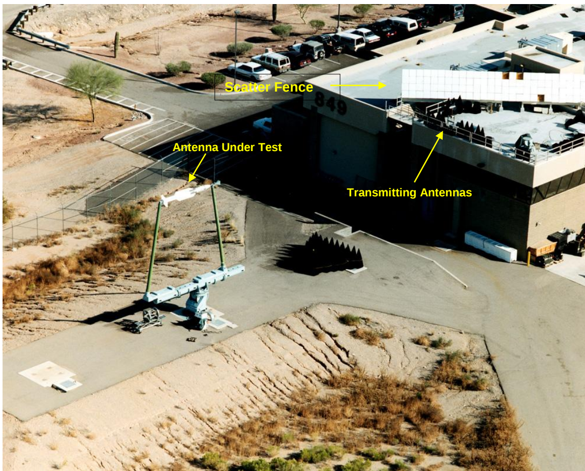
Figure 2: Outdoor Antenna Test Range
